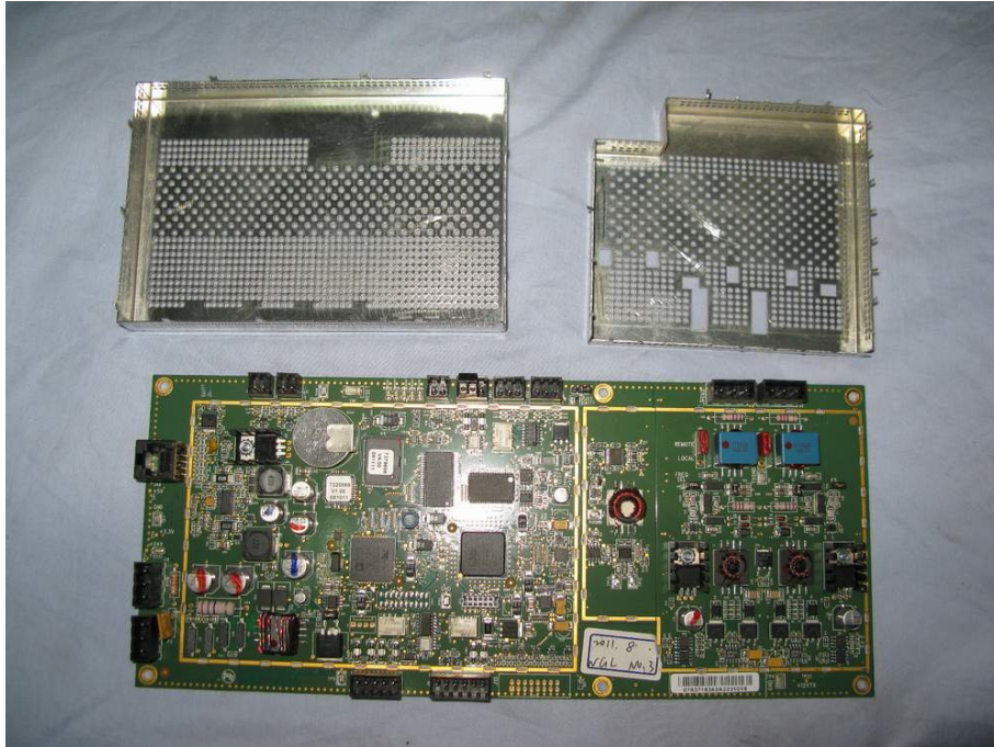
PCB 3 View2 (without shielding)
