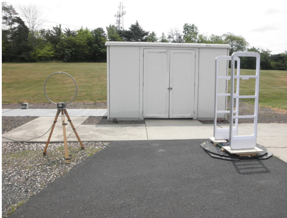
Perpendicular Antenna Polarization, Below 30 MHz
