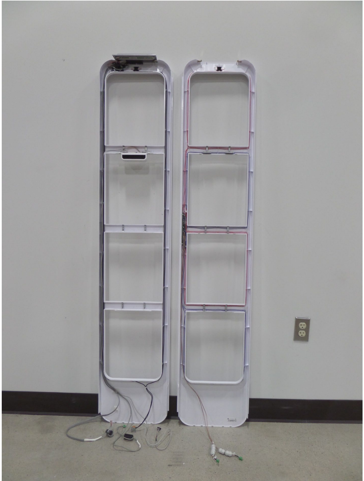
Figure 1: NP22 PRI/PAB/SAB RF ANT FRAME TWO HALVES
