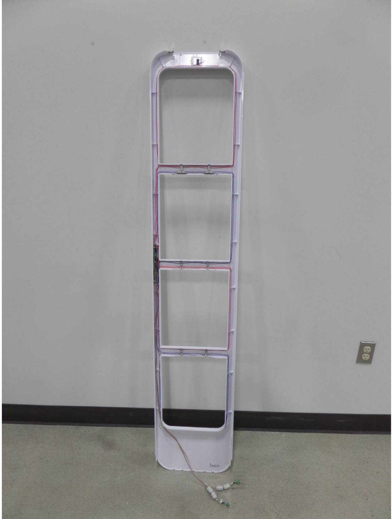
Figure 2: NP22 PRI/PAB/SAB RF ANT FRAME BACK SIDE
