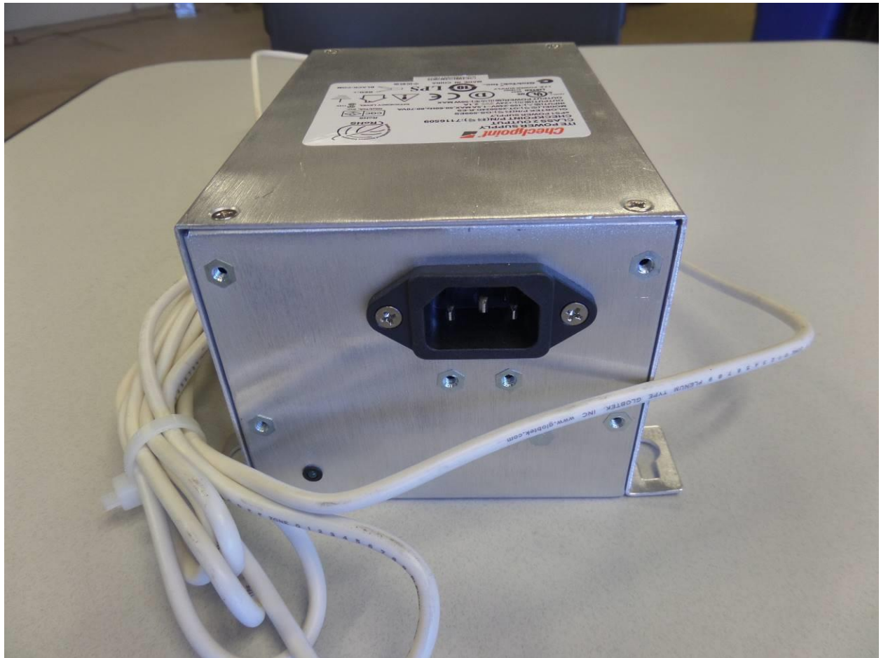
Photograph 15. Globtek 50W PS top side
