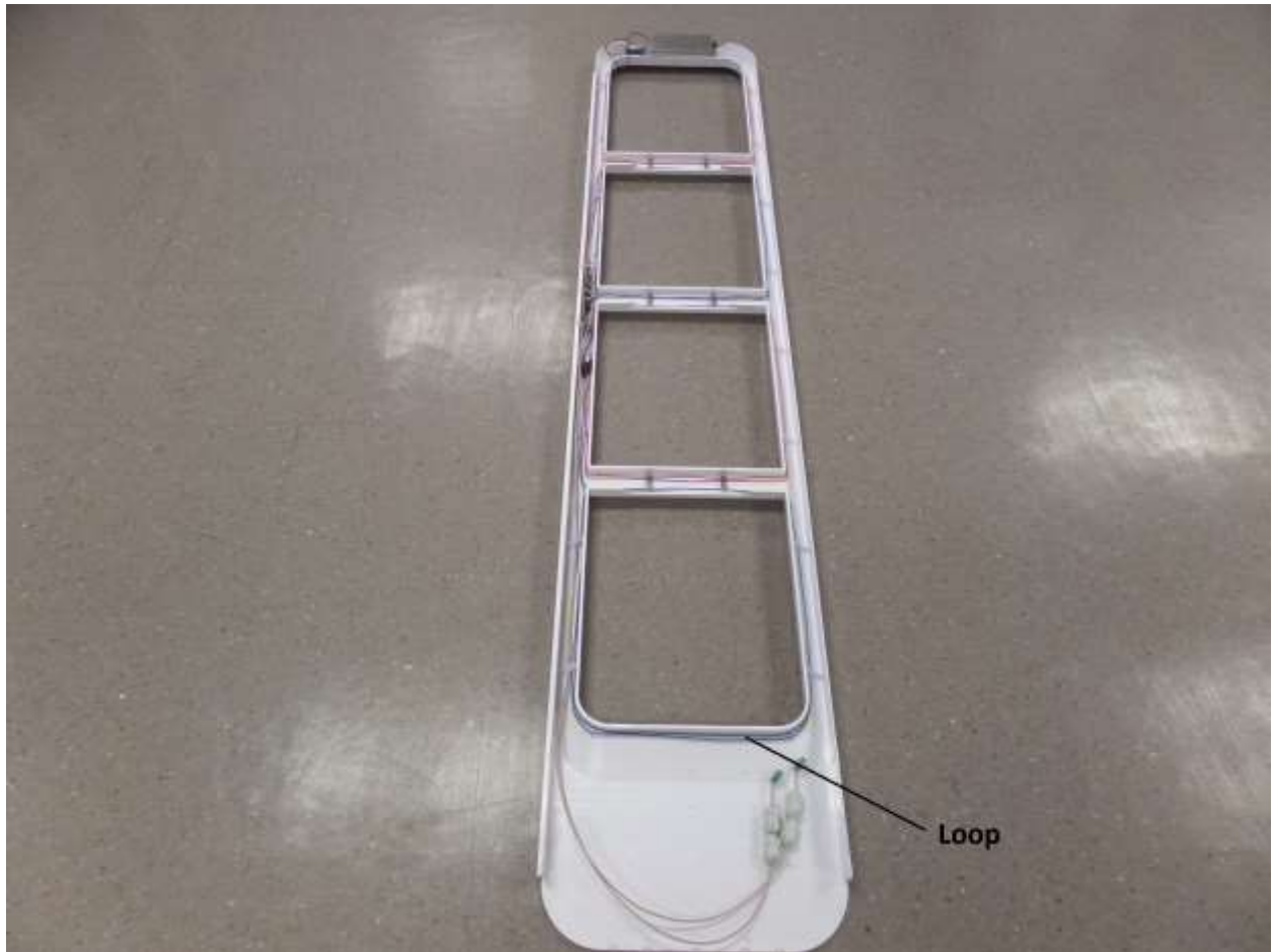
NP20 top side split view pointing out loop
