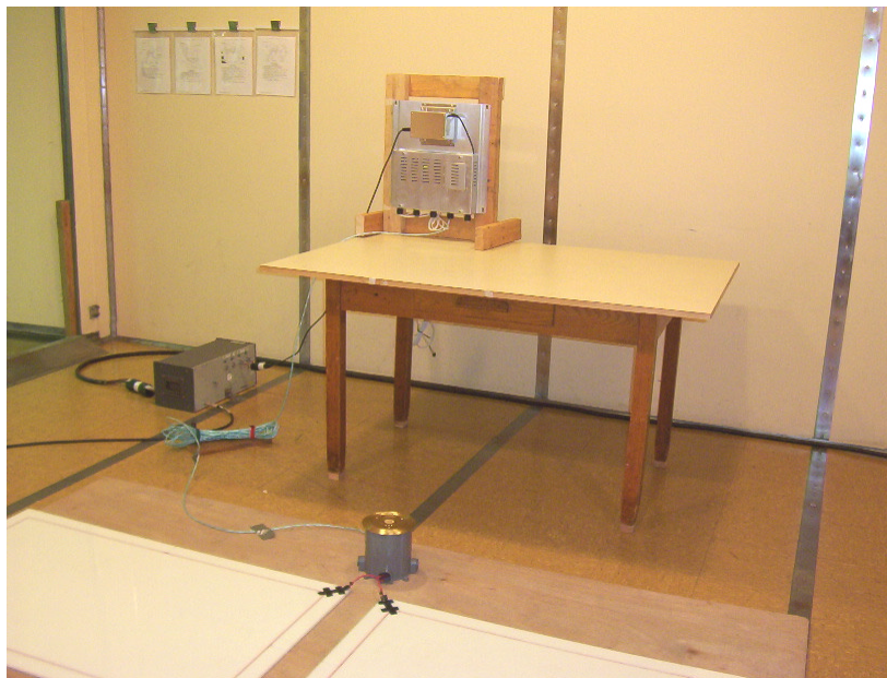
Photo: Liberty FX – Unshielded, Conducted Emissions Test Setup
