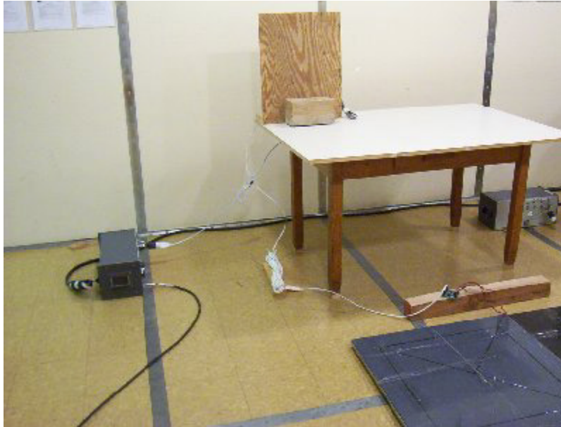
Photo: Liberty FX – Shielded, Conducted Emissions Test Setup
