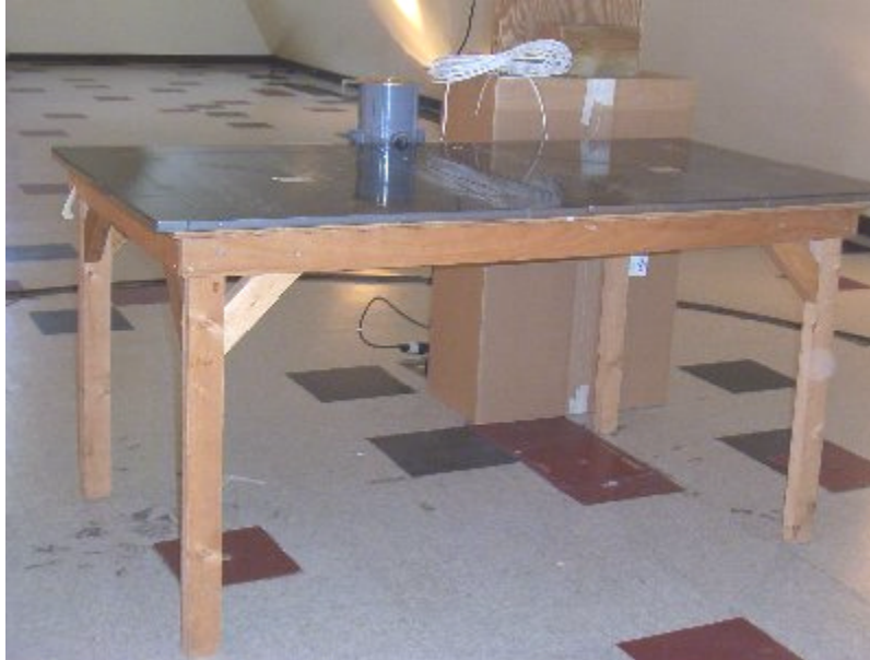
Photo: Liberty FX – Shielded, Radiated Emissions, Front View (50' antenna transmission line bundle placed on box for maximum emission)
