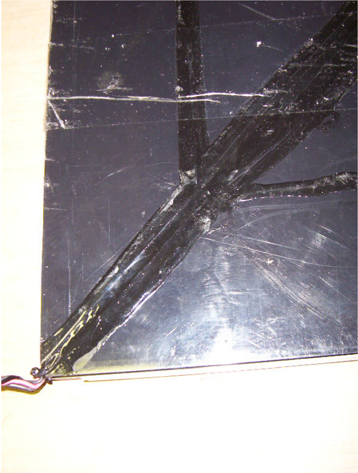
Liberty FX Shielded Antenna Panel (close up of wire and seal)
