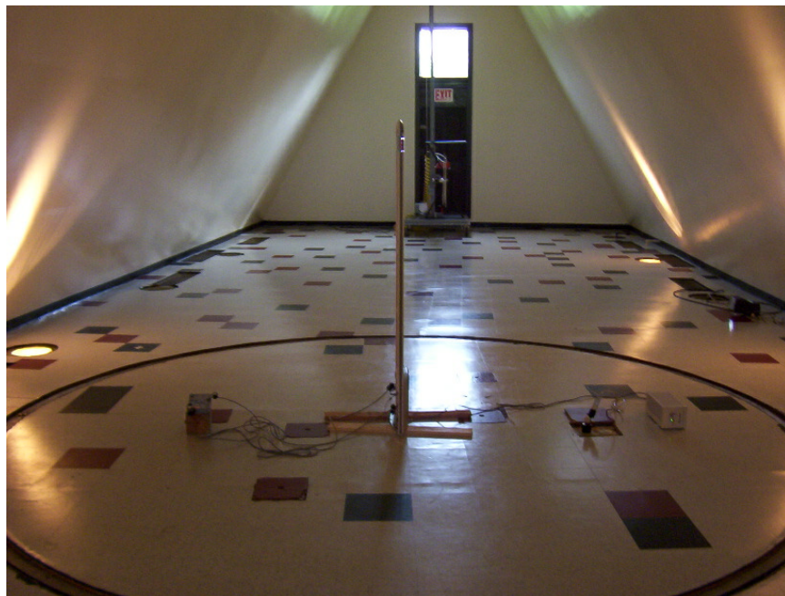
Photo 3 – Photo of EMI Test Setup (Front View)
