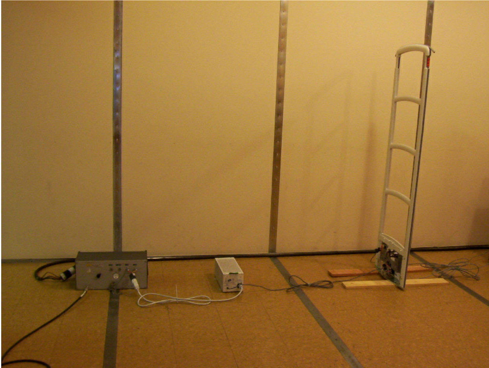
Photo 1 – LIBERTY DX – CONDUCTED EMISSIONS TEST SETUP
