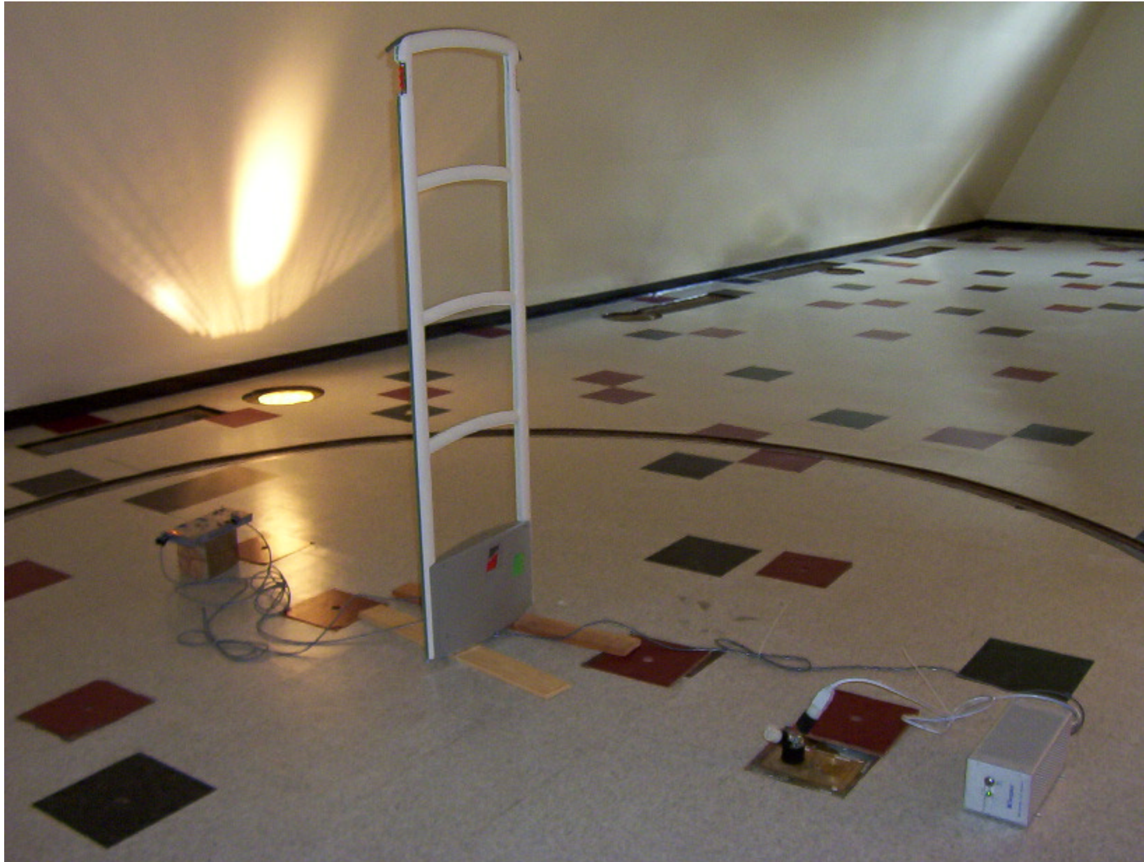
PHOTO 3 – LIBERTY DX SIDE VIEW OF RADIATED EMISSIONS TEST SETUP
