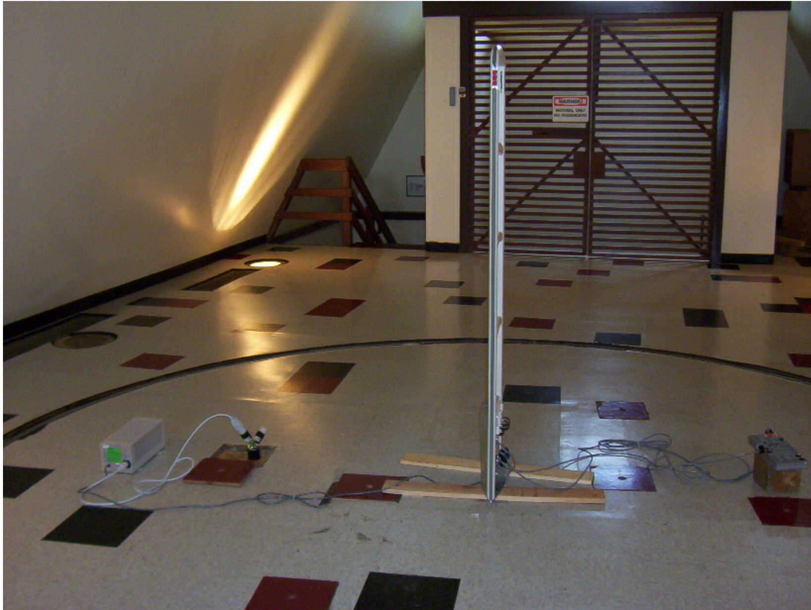
PHOTO 2 – LIBERTY DX REAR VIEW OF RADIATED EMISSIONS TEST SETUP
