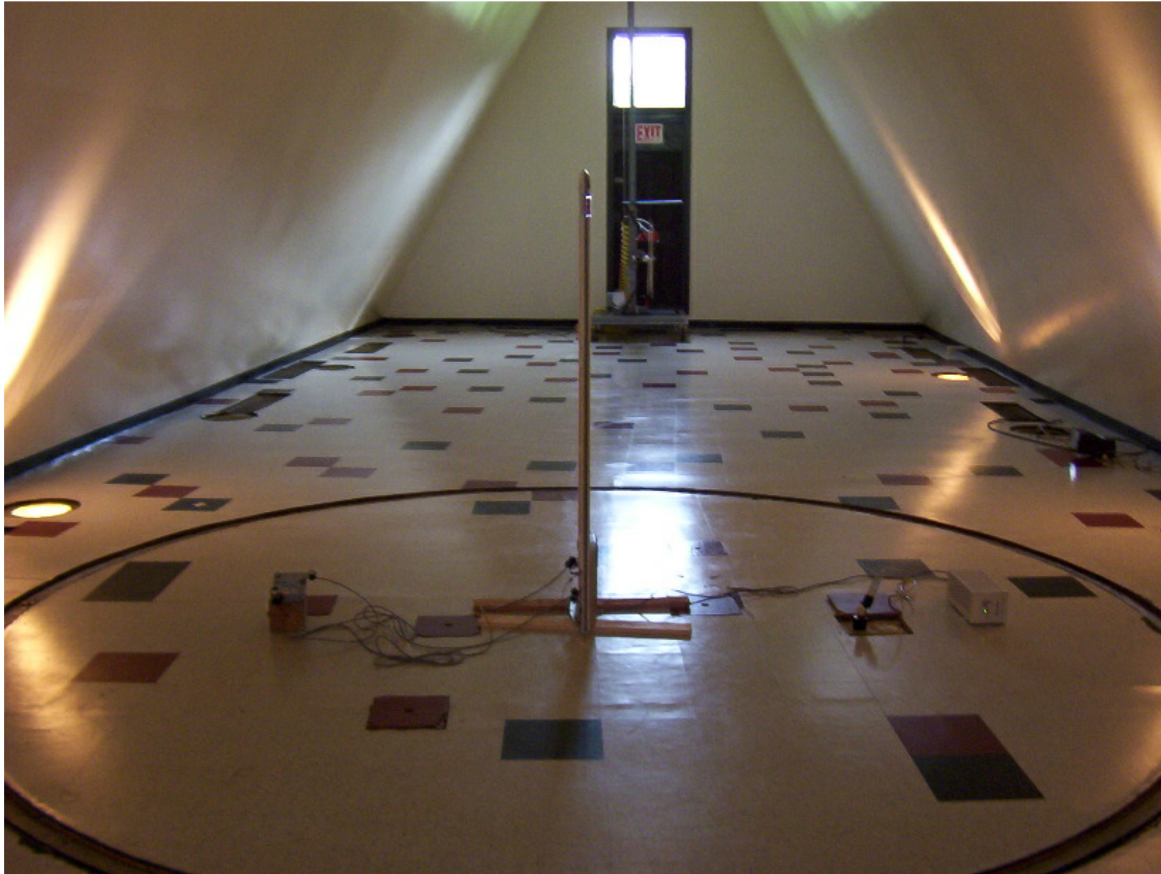
PHOTO 1 – LIBERTY DX FRONT VIEW OF TEST SETUP FOR REDIATED EMISSIONS
