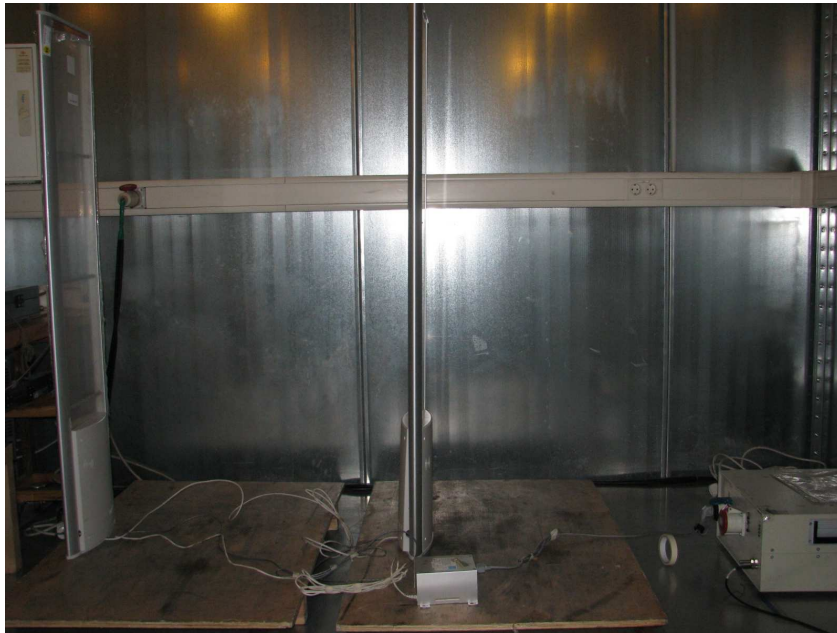
Photograph 2: Set-up for radiated emission (9kHz - 30MHz)
