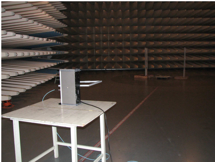
Photograph 2: Set-up for radiated emission (9kHz - 30MHz)
