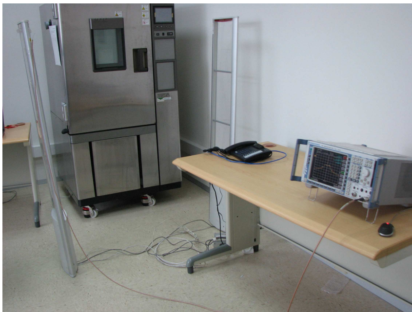
Photograph 4: Set-up for emission bandwidth & duty cycle
