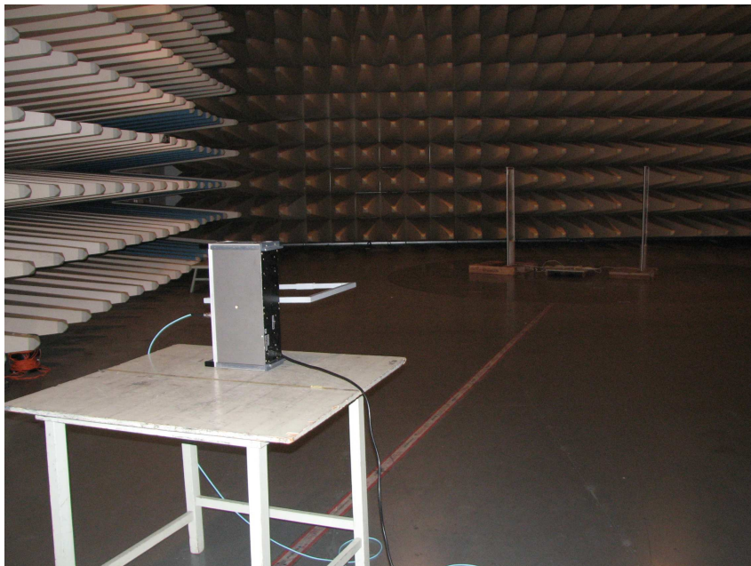
Photograph 2: Set-up for radiated emission (9kHz - 30MHz)
