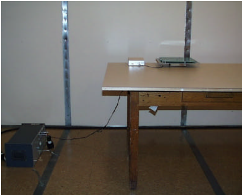
Photo 5 – Conducted Emissions Test Setup – Front View
