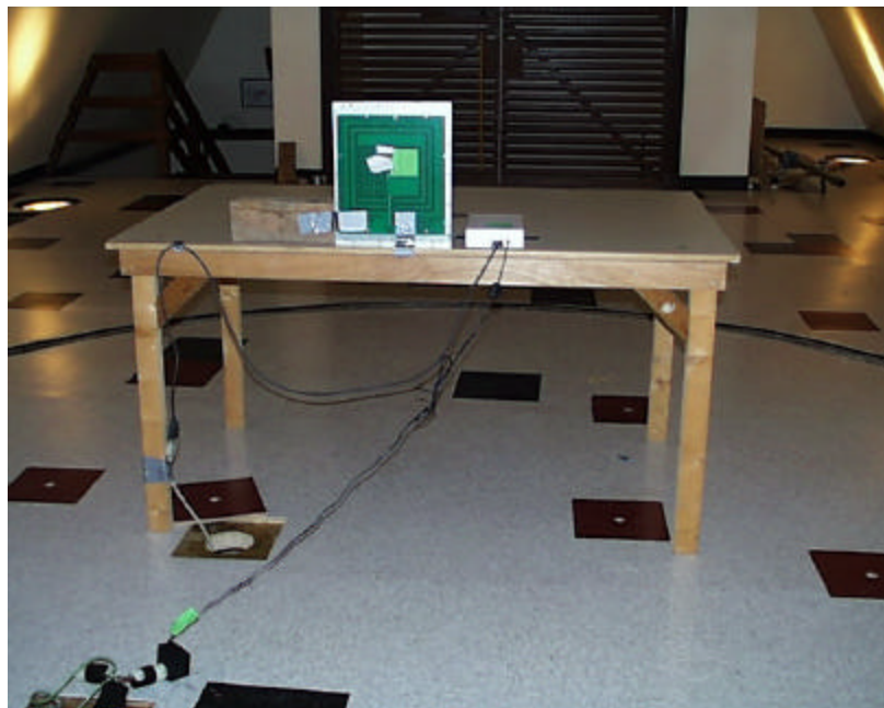
Photo 4 – Radiated Emissions Test Setup – Rear View
