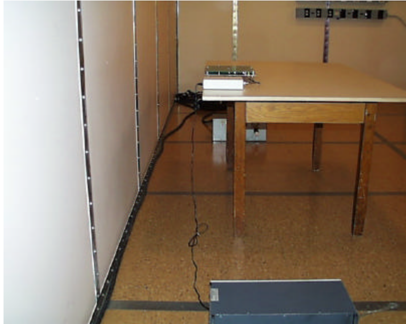
Photo 6 – Conducted Emissions Test Setup – Front View
