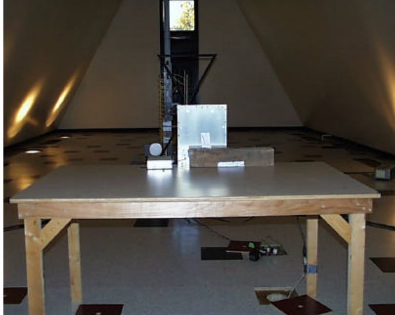
Photo 3 – Radiated Emissions Test Setup – Front View
