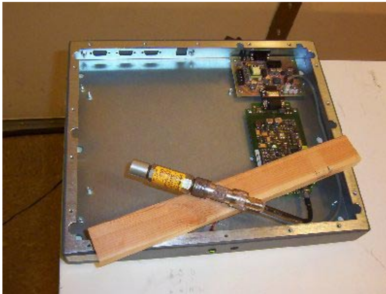
Staff Station Reader (Serial Version): 50-ohm load on transmitter
