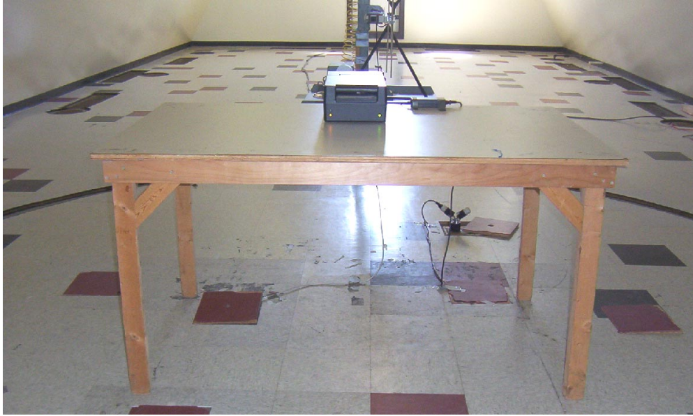
Radiated Emission Test Setup (Front)
