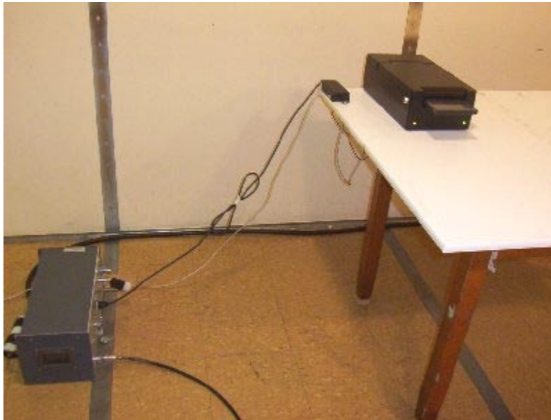
ISO ILS IUS: Conducted Emission Test Setup
