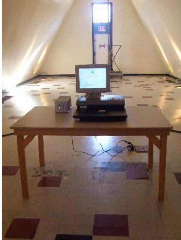
Radiated Emissions Test Setup Front
