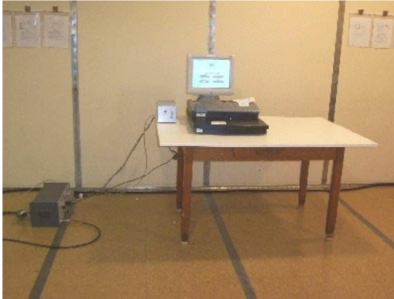
ISO ILS Open Plus Patron Self Checkout Station: Conducted Emission Test Setup
