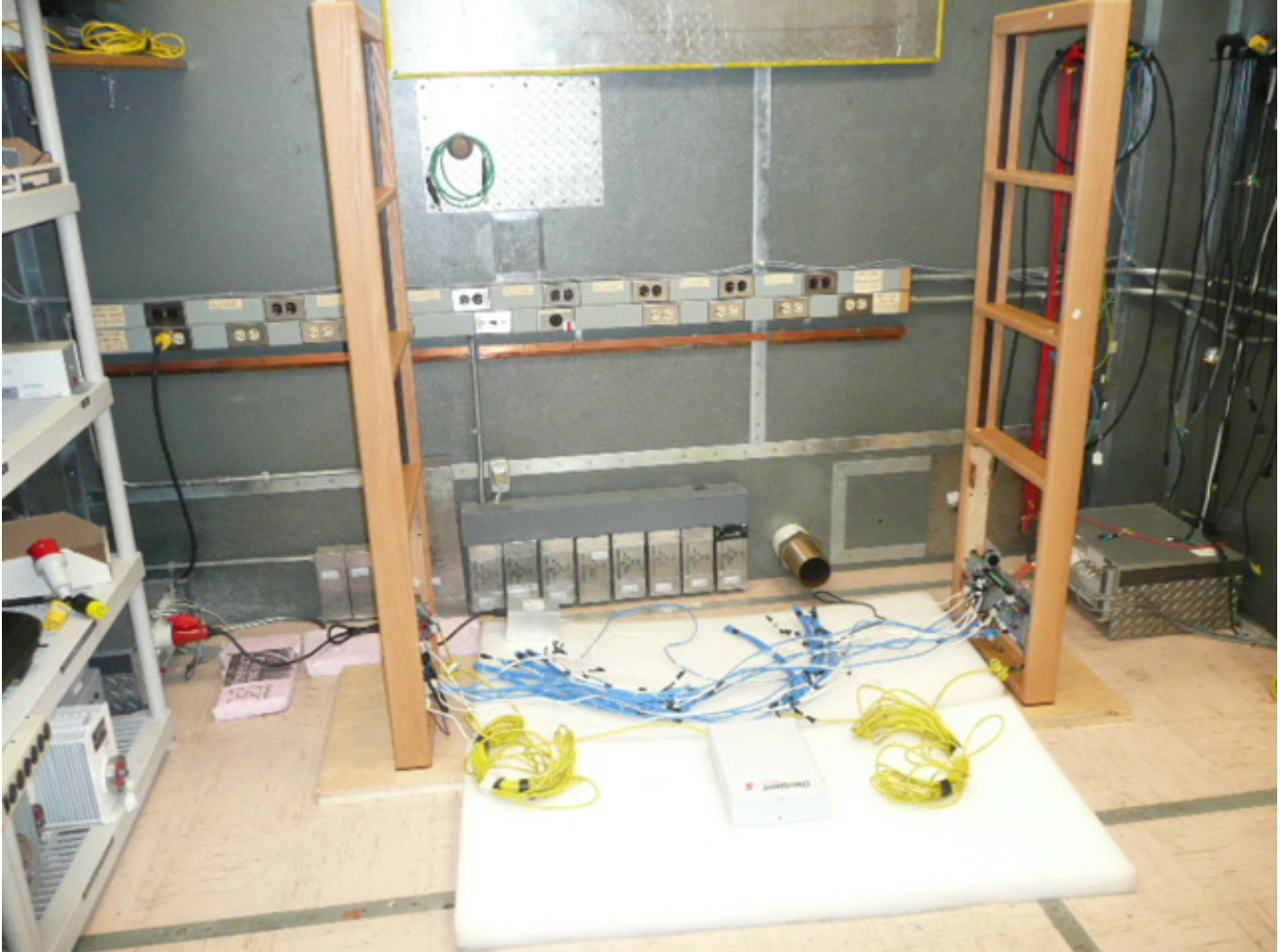
Figure 3 – Conducted Emissions Test Setup
