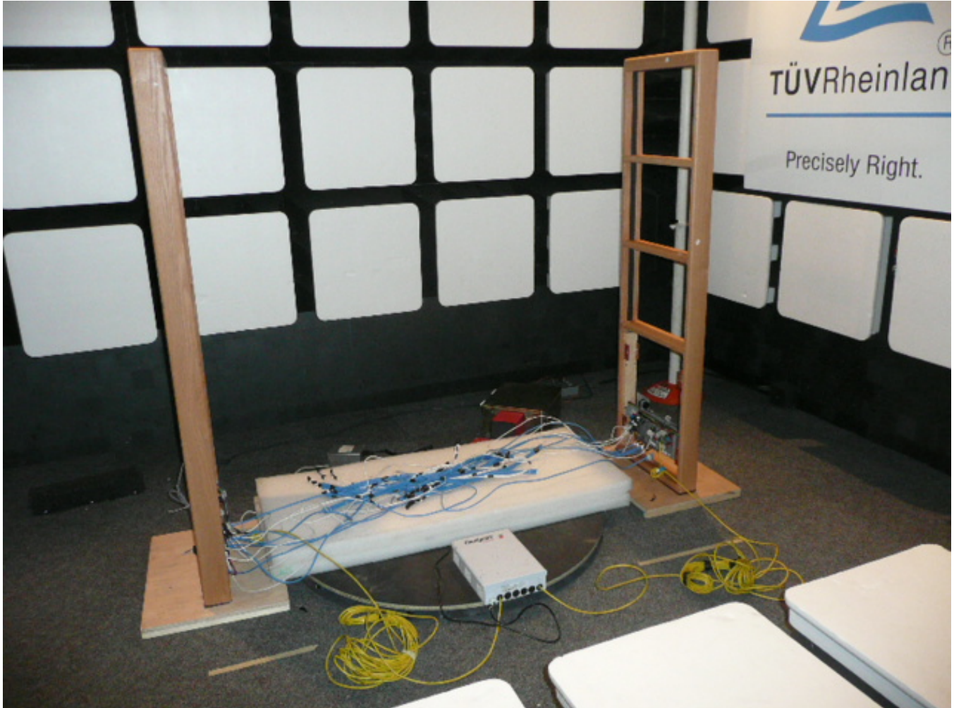
Figure 1 - Radiated Emissions Test Setup (Semi-Anechoic Chamber)
