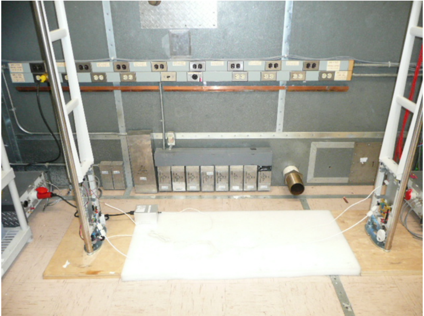
Figure 6 – Conducted Emissions Test Setup – P-10
