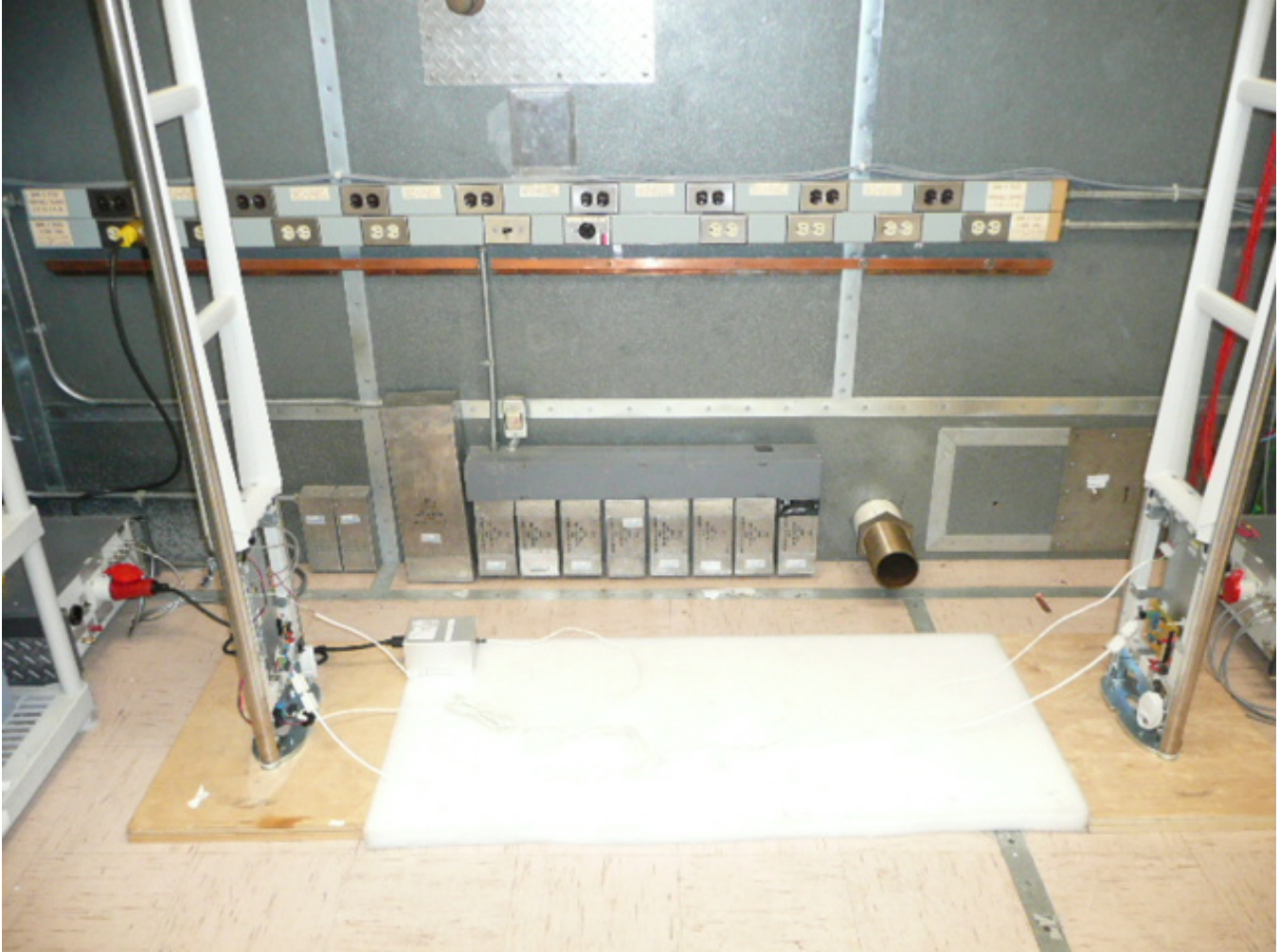
Figure 5 – Conducted Emissions Test Setup – P-20
