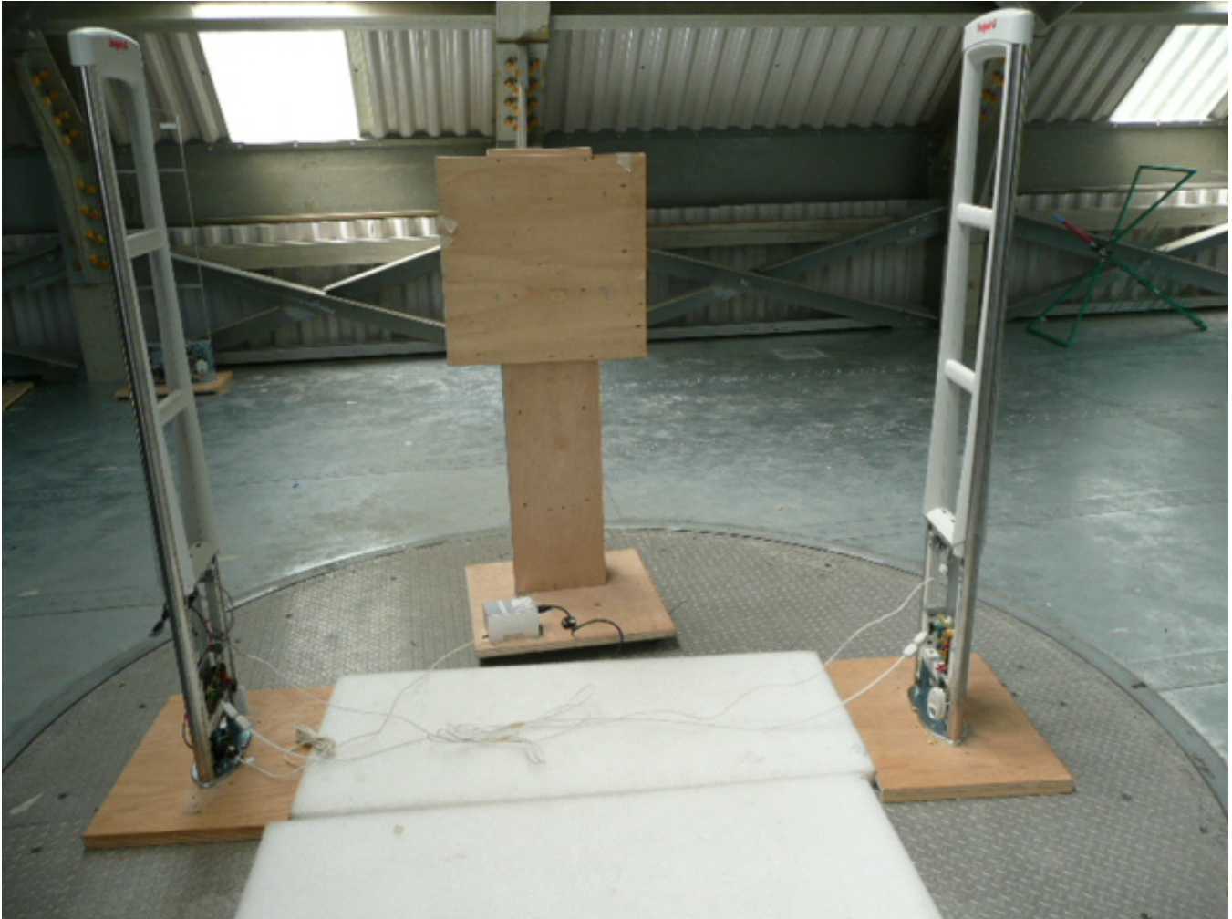
Figure 1 – Radiated Emissions Test Setup – P-20
