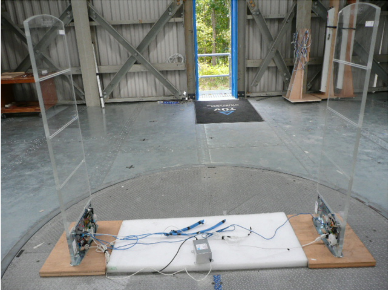
Figure 4 – Radiated Emissions Test Setup – G-10
