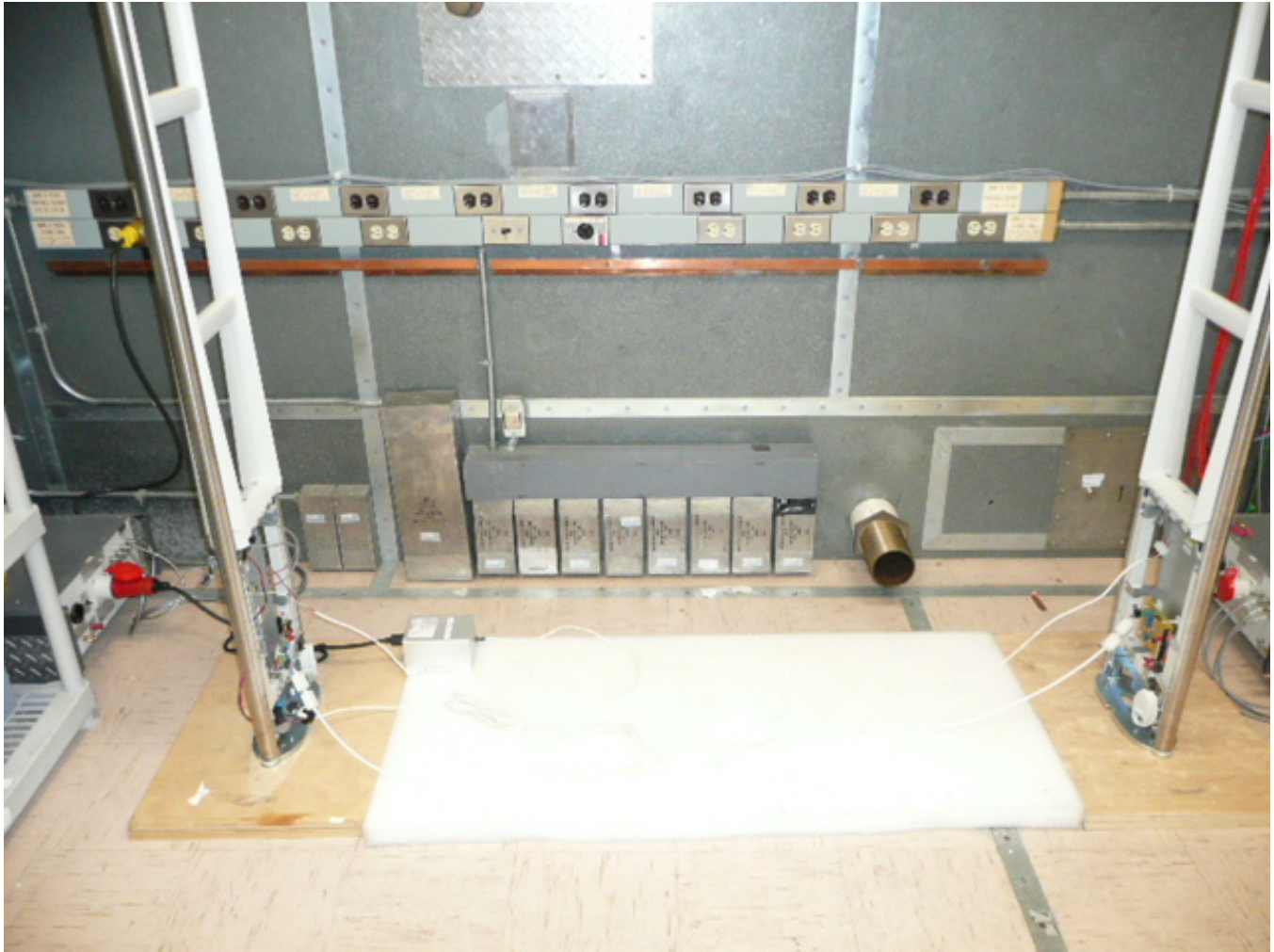
Figure 12 – Conducted Emissions Test Setup – P-10
