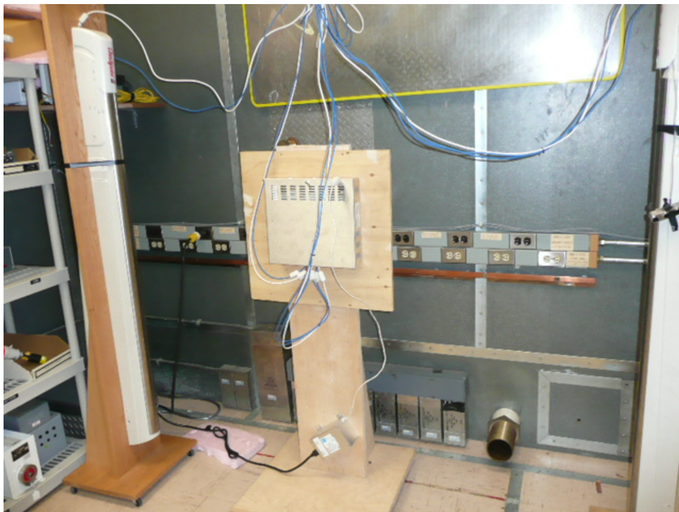
Figure 15 – Conducted Emissions Test Setup – S-10
