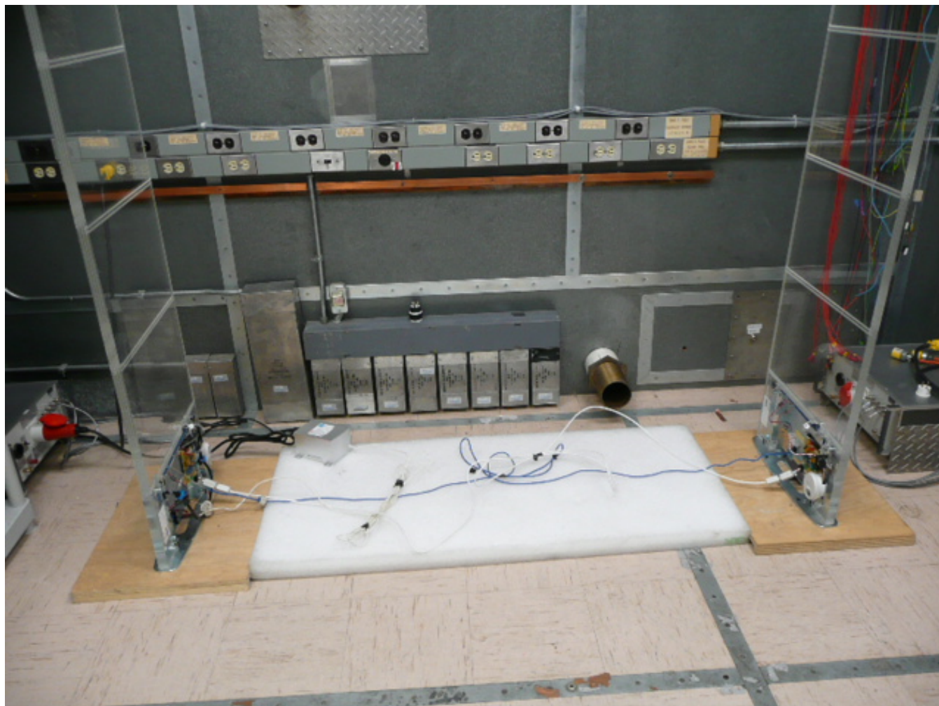
Figure 14 – Conducted Emissions Test Setup – G-10
