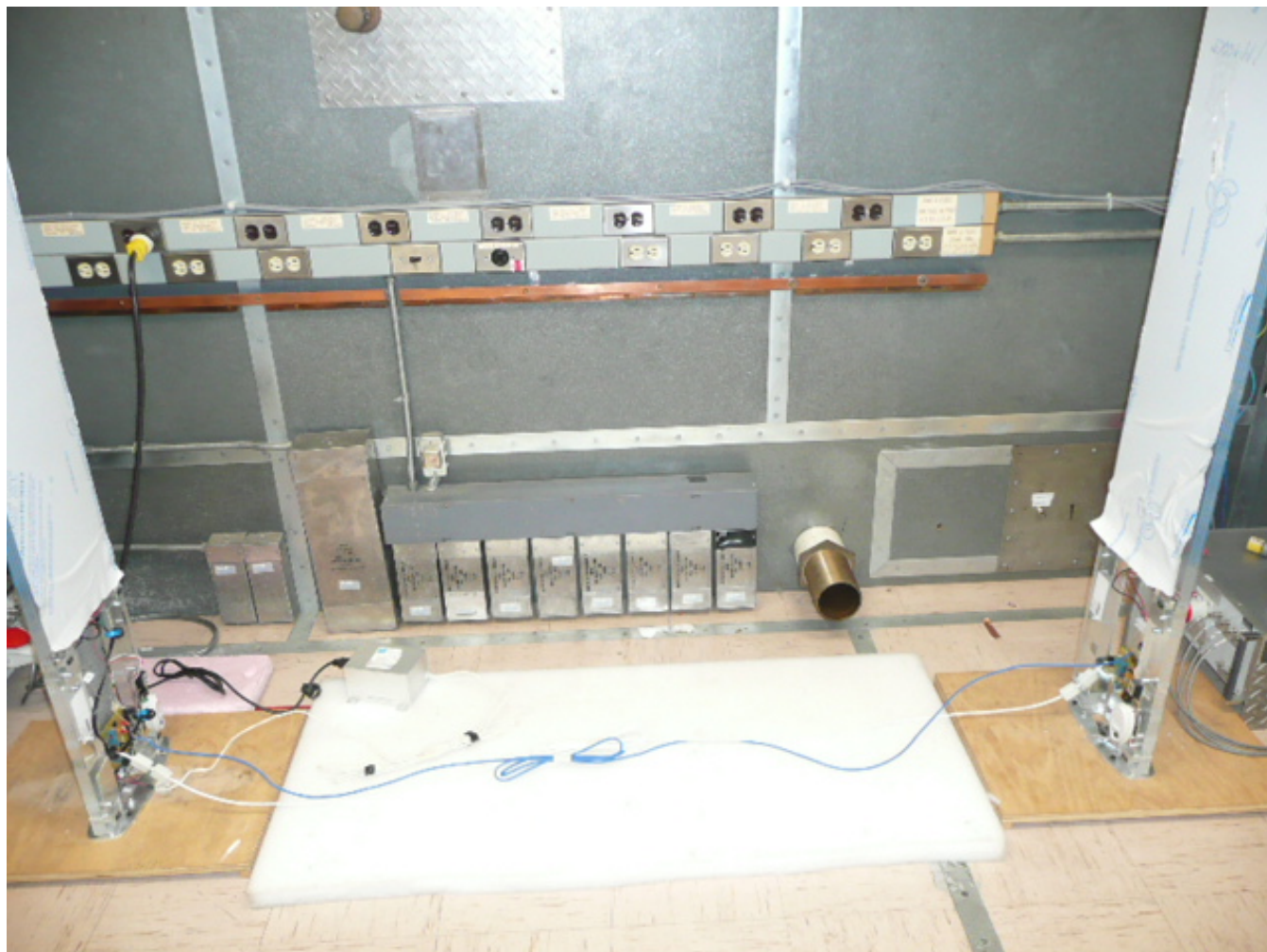
Figure 13 – Conducted Emissions Test Setup – G-20
