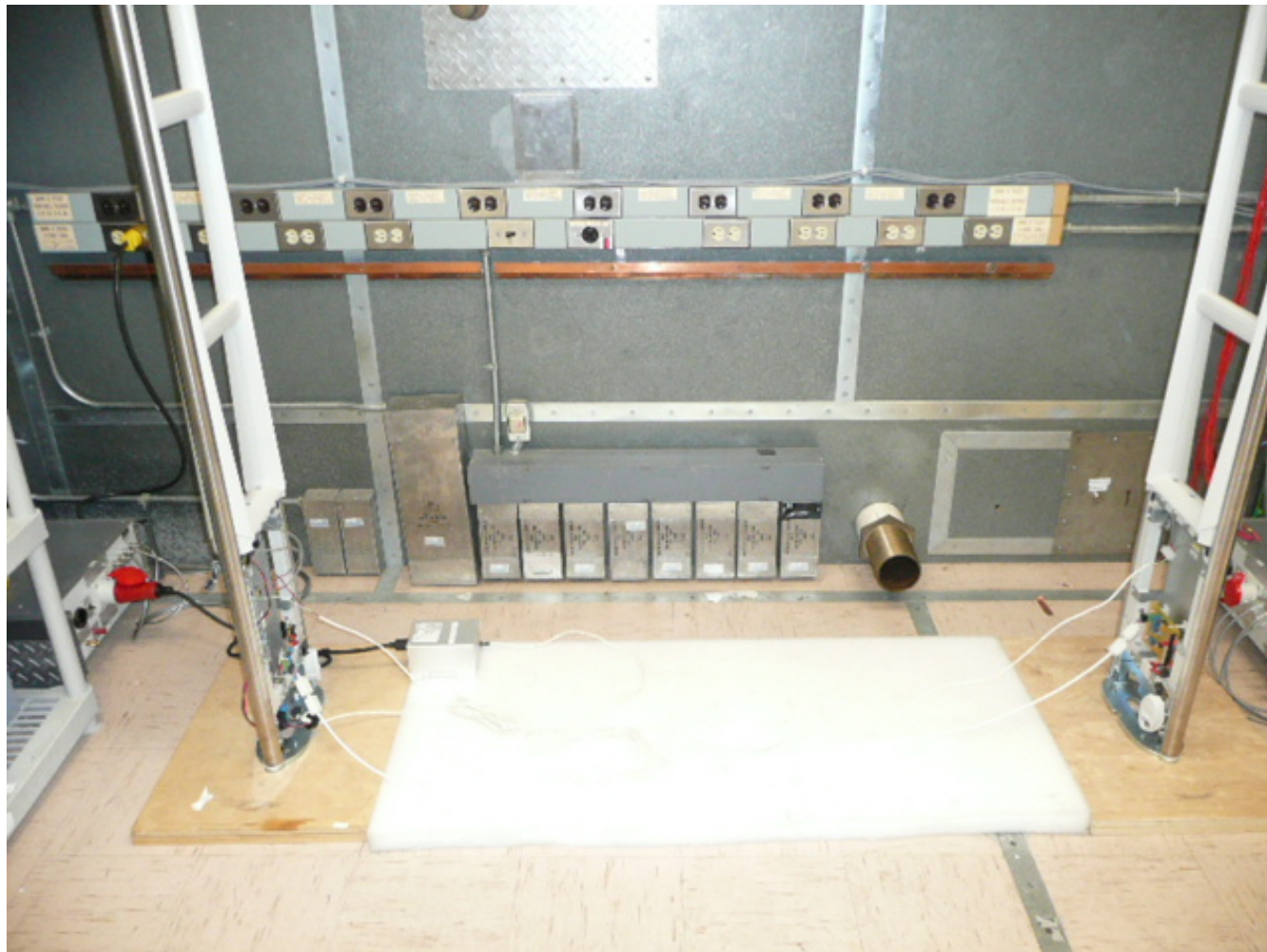
Figure 11 – Conducted Emissions Test Setup – P-20
