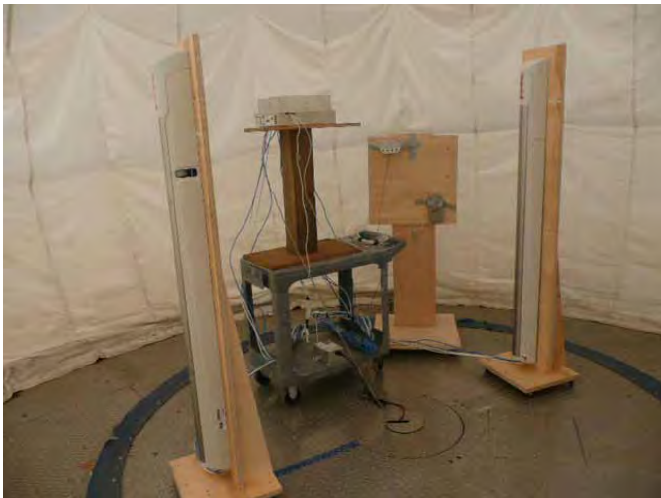
Figure 17 - Radiated Emissions (3m OATS) Test Setup. Configuration 1
