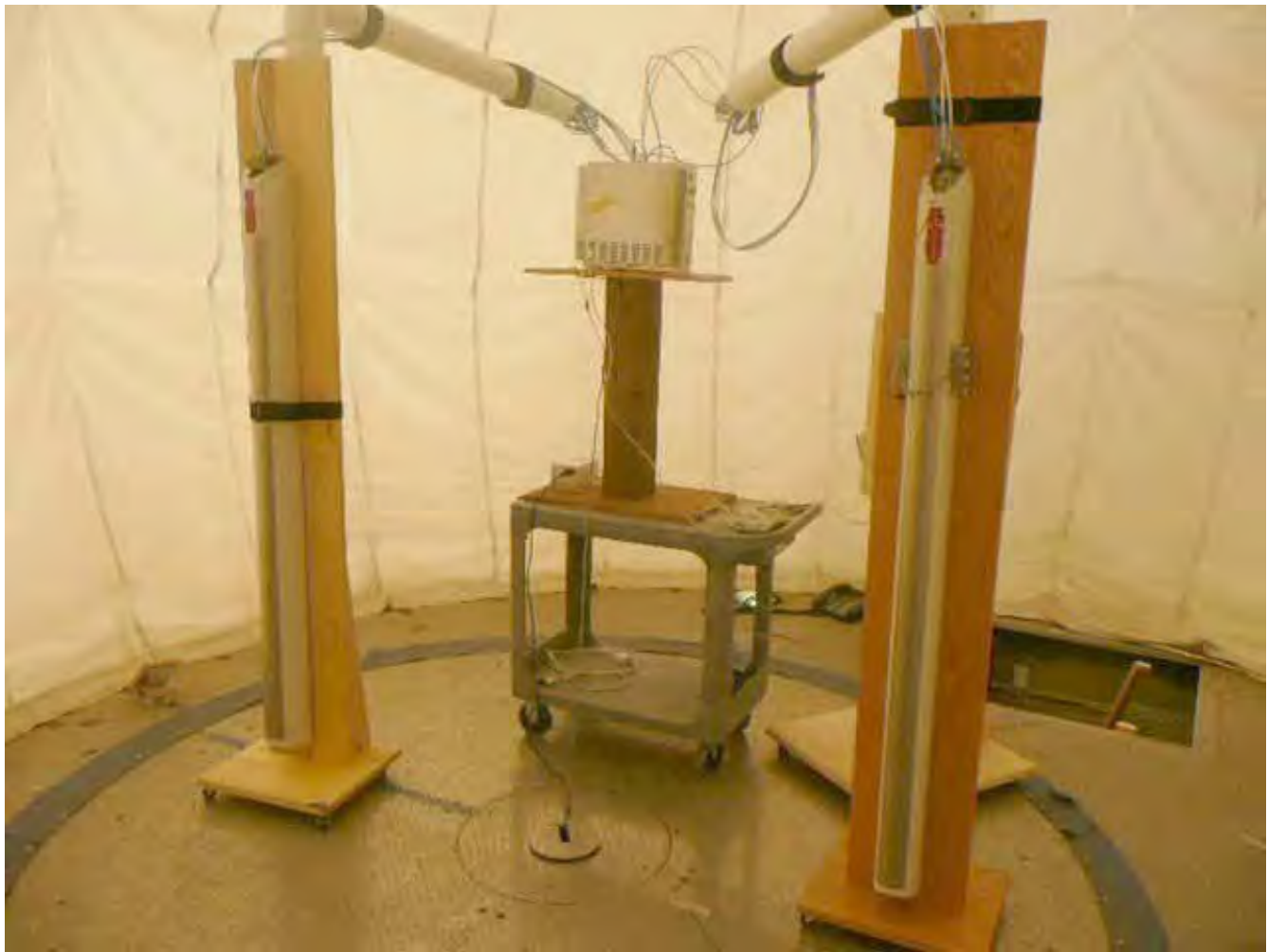
Figure 19 - Radiated Emissions (3m OATS) Test Setup. Configuration 2
