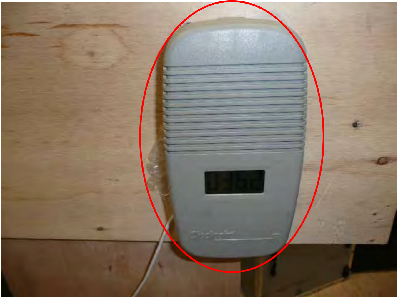
Figure 8 –EAS Voice alarm Configuration 1 and 2
