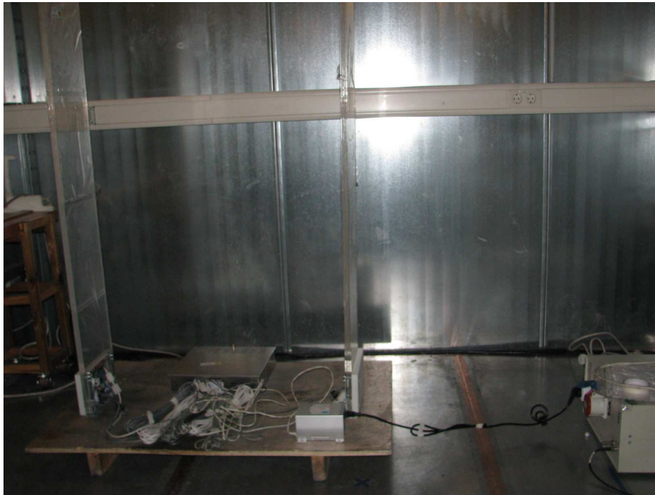
Photograph 2: Set-up for radiated emission (9kHz - 30MHz)
