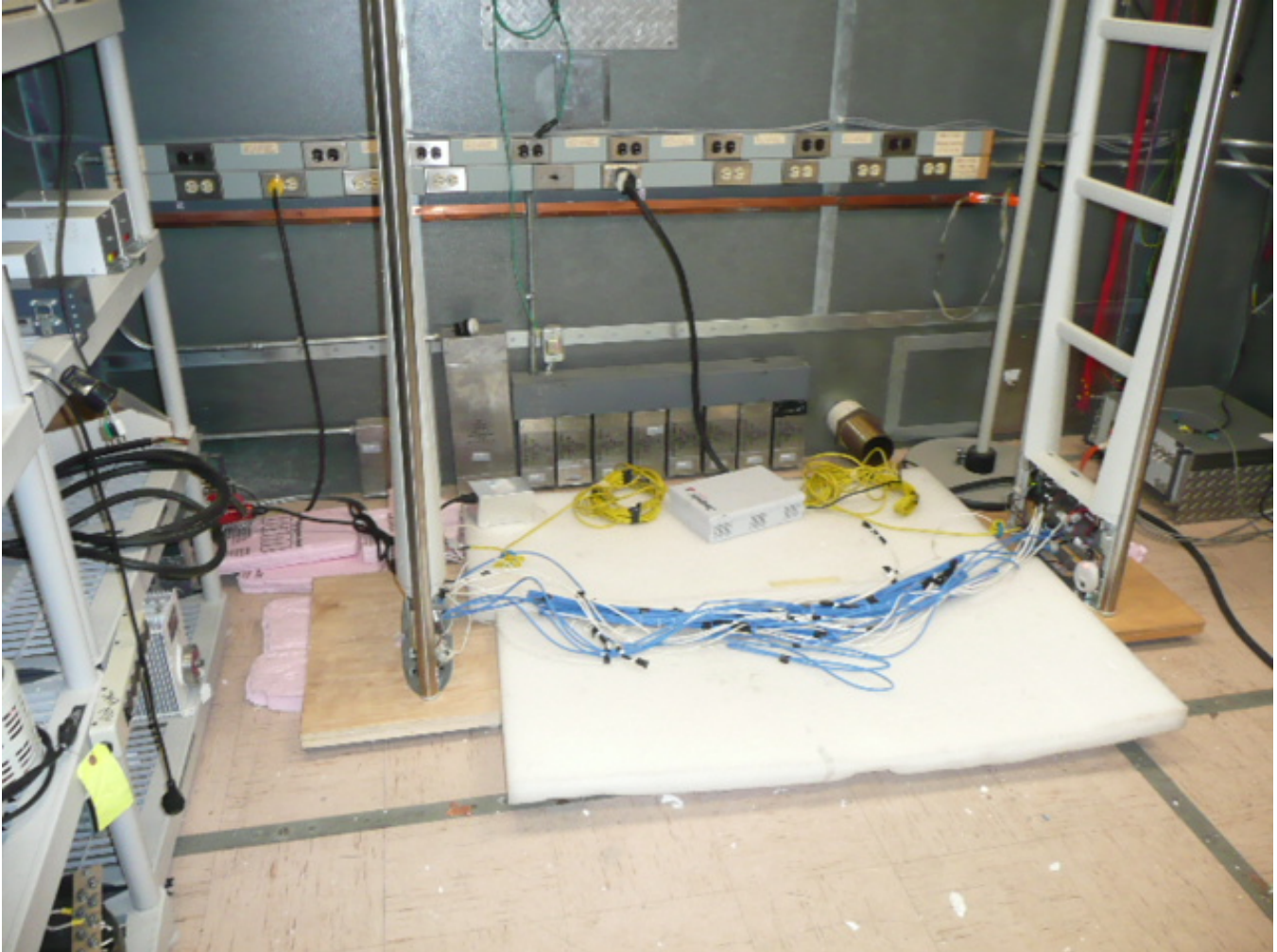
Figure 5 – Conducted Emissions Test Setup – P-10
