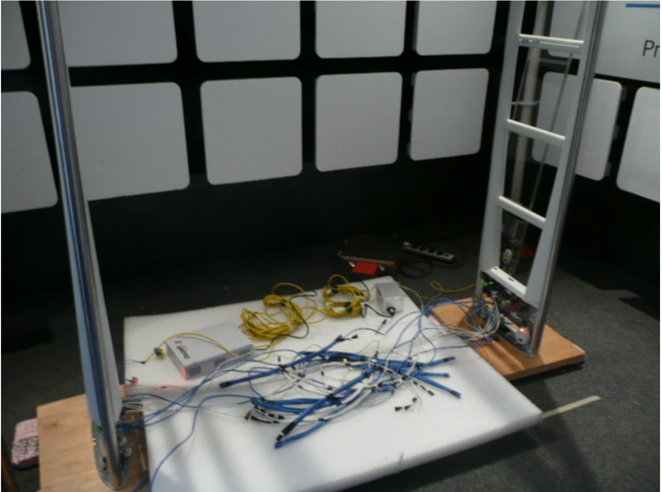
Figure 1 - Radiated Emissions Test Setup (Semi-Anechoic Chamber) – P-10
