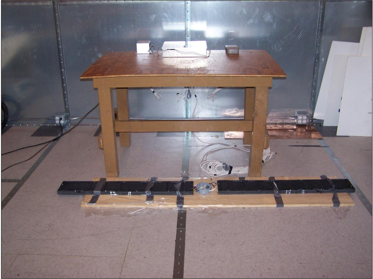
Photograph 3. Conducted Emissions, 15.207(a), Test Setup
