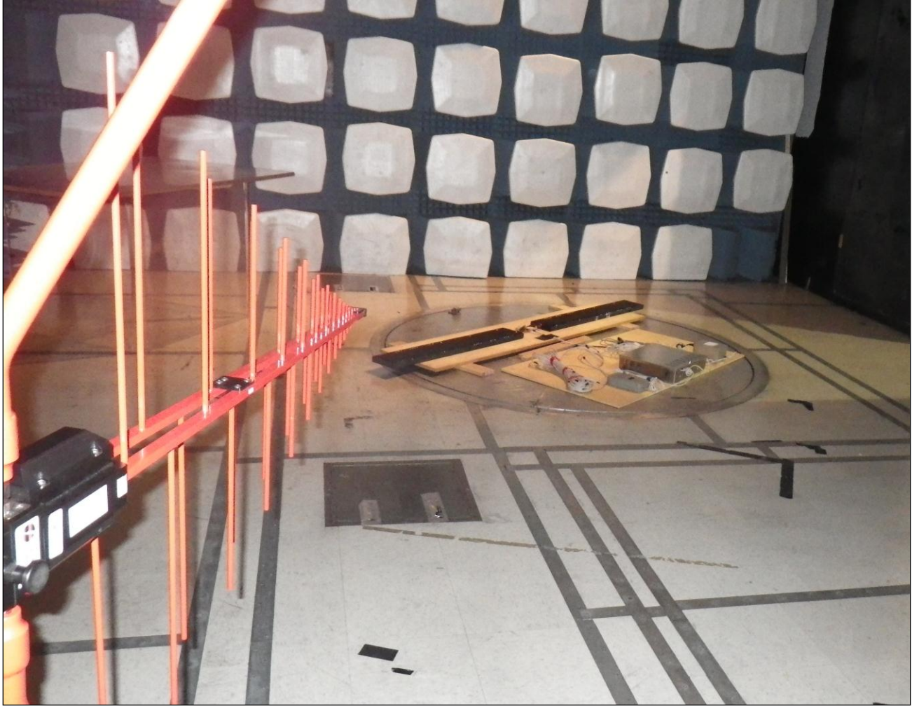
Photograph 2. Radiated Emission, Test Setup
