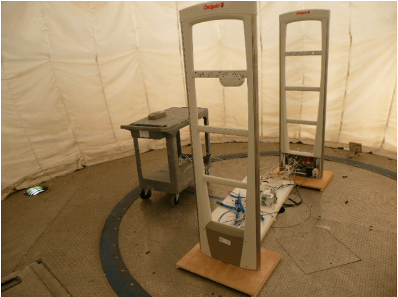
Figure 25 – Radiated Emissions (3m OATS) and Harmonics of Fundamental Emissions Test Setup (10m OATS) P10 Configuration 1
