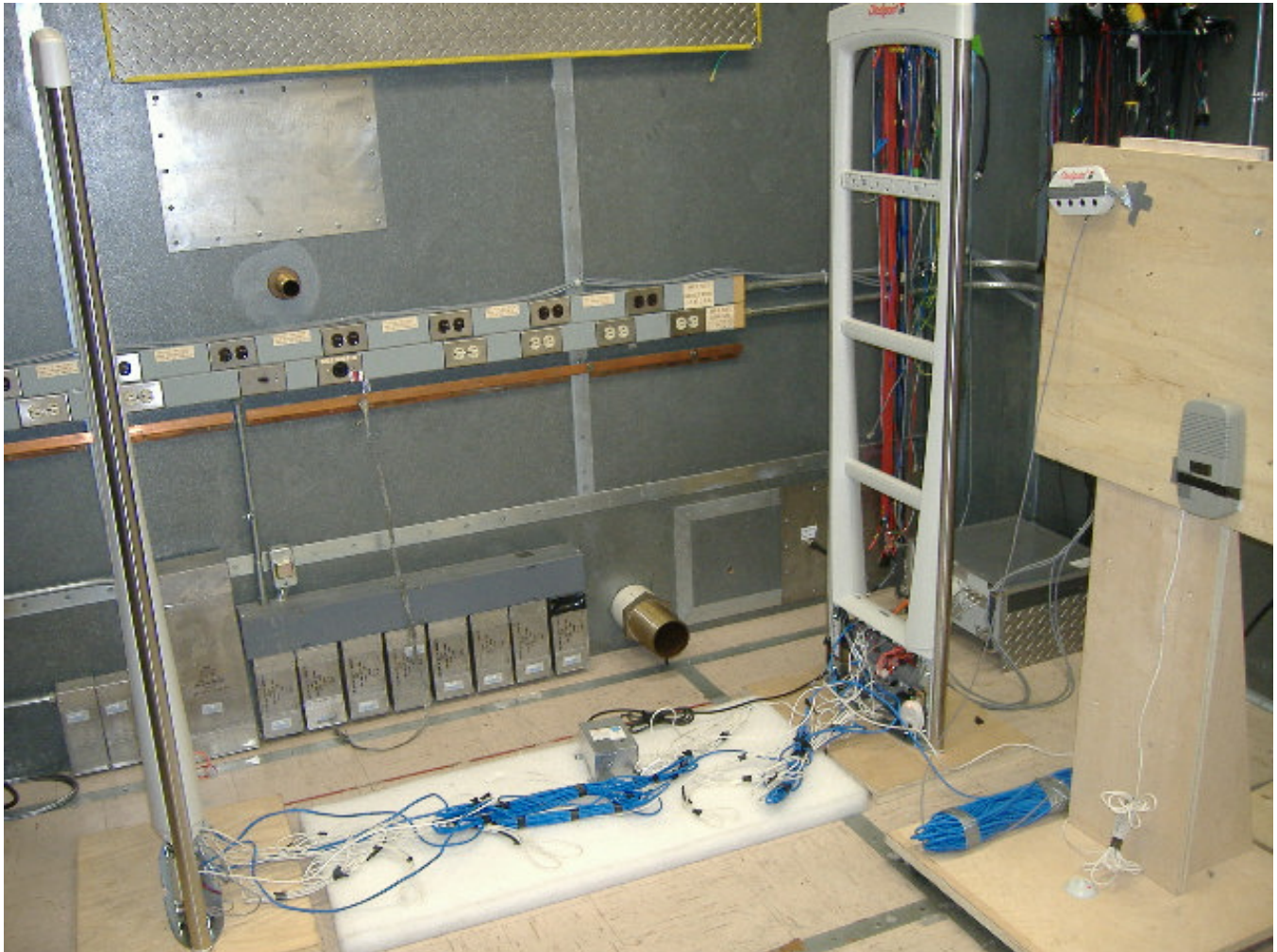
Figure 22 –Conducted Emissions Test Setup P10. Configuration 2
