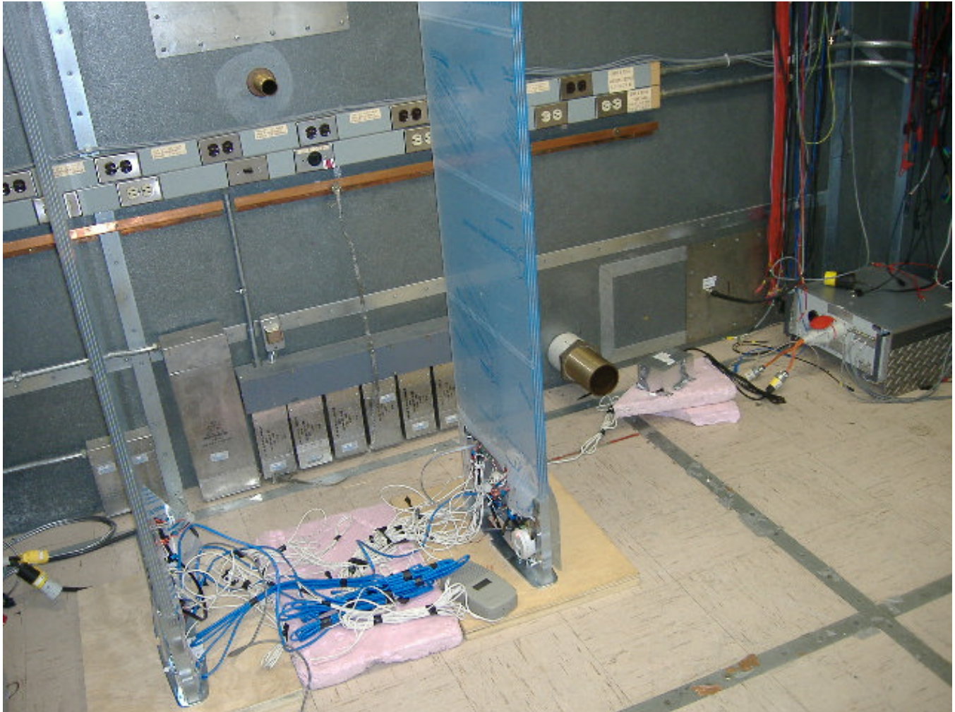
Figure 20 –Conducted Emissions Test Setup G10 Configuration 1
