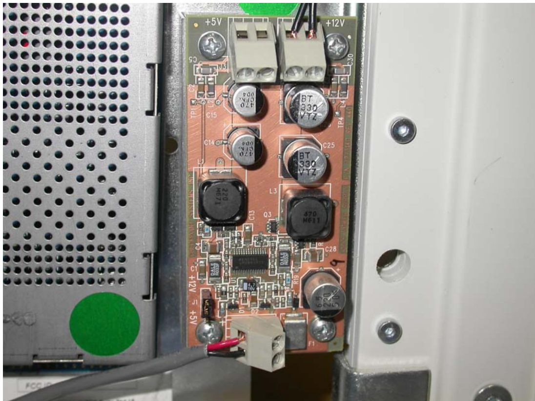
DC power supply for CB 3000
