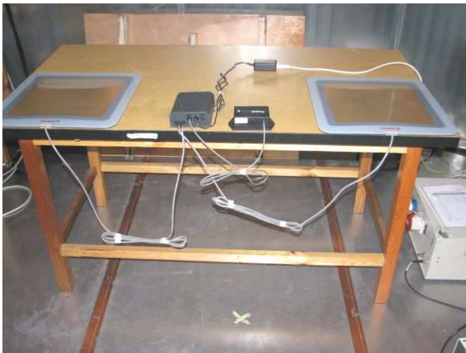
Photograph 3: Set-up for conducted emission
