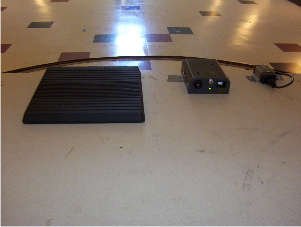
Checkpoint Systems, Inc.: CP9-2 Radiated Emissions Test Setup Photo (Front View)
