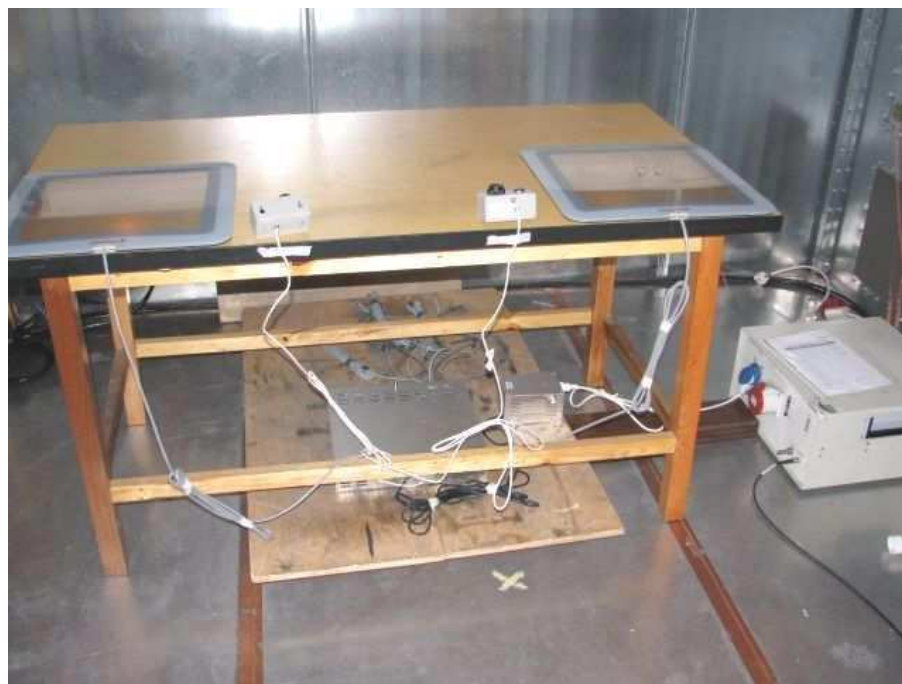
Photograph 3: Set-up for conducted emission
