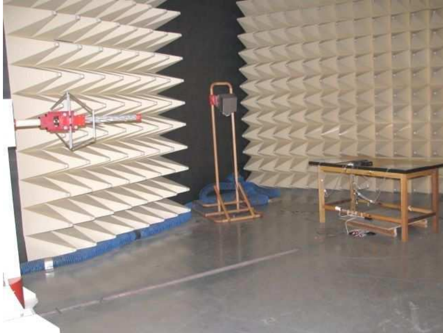
Photograph 5: Set-up for radiated emission (30 - 1000MHz)
