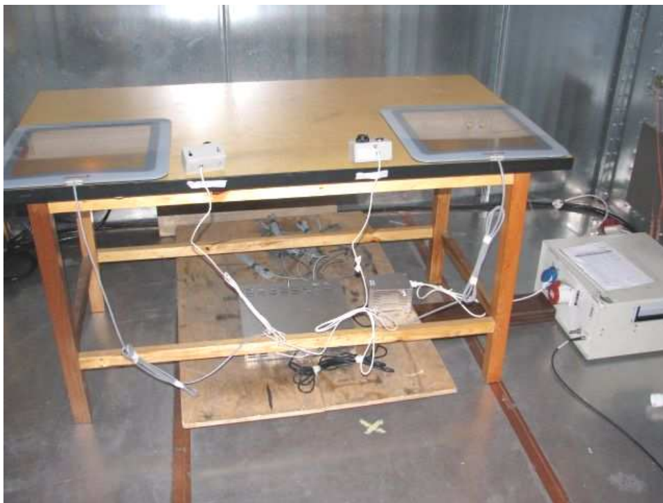
Photograph 3: Set-up for conducted emission
