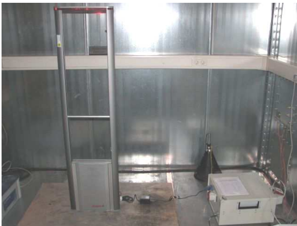
Photograph 2: Set-up for radiated emission (9kHz - 30MHz)
