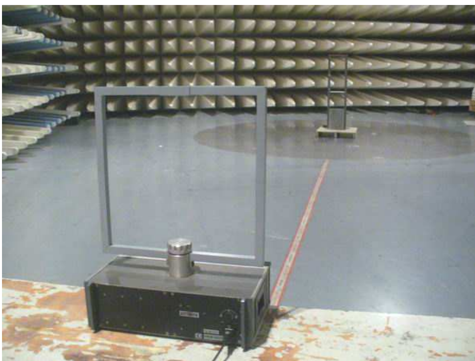
Photograph 2: Set-up for radiated emission (9kHz - 30MHz)
