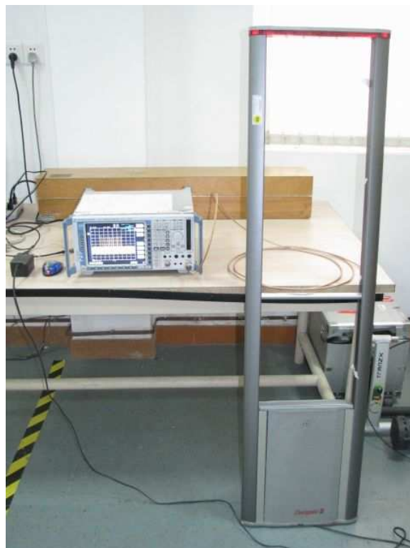
Photograph 4: Set-up for emission bandwidth & duty cycle
