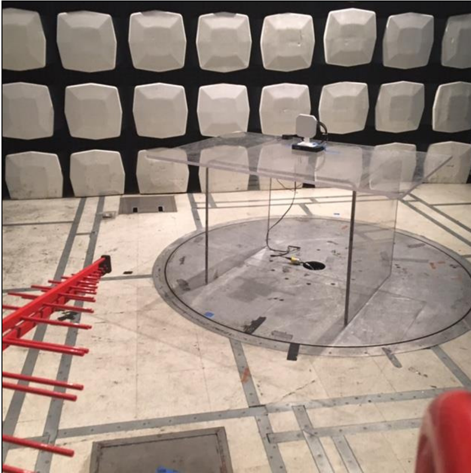
Photograph 2. Radiated Spurious Emissions, Test Setup
