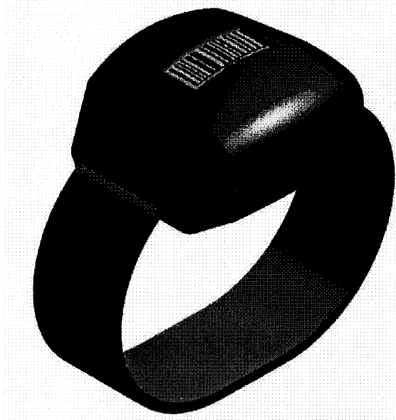
Figure 1: PASS Transmitter Unit
