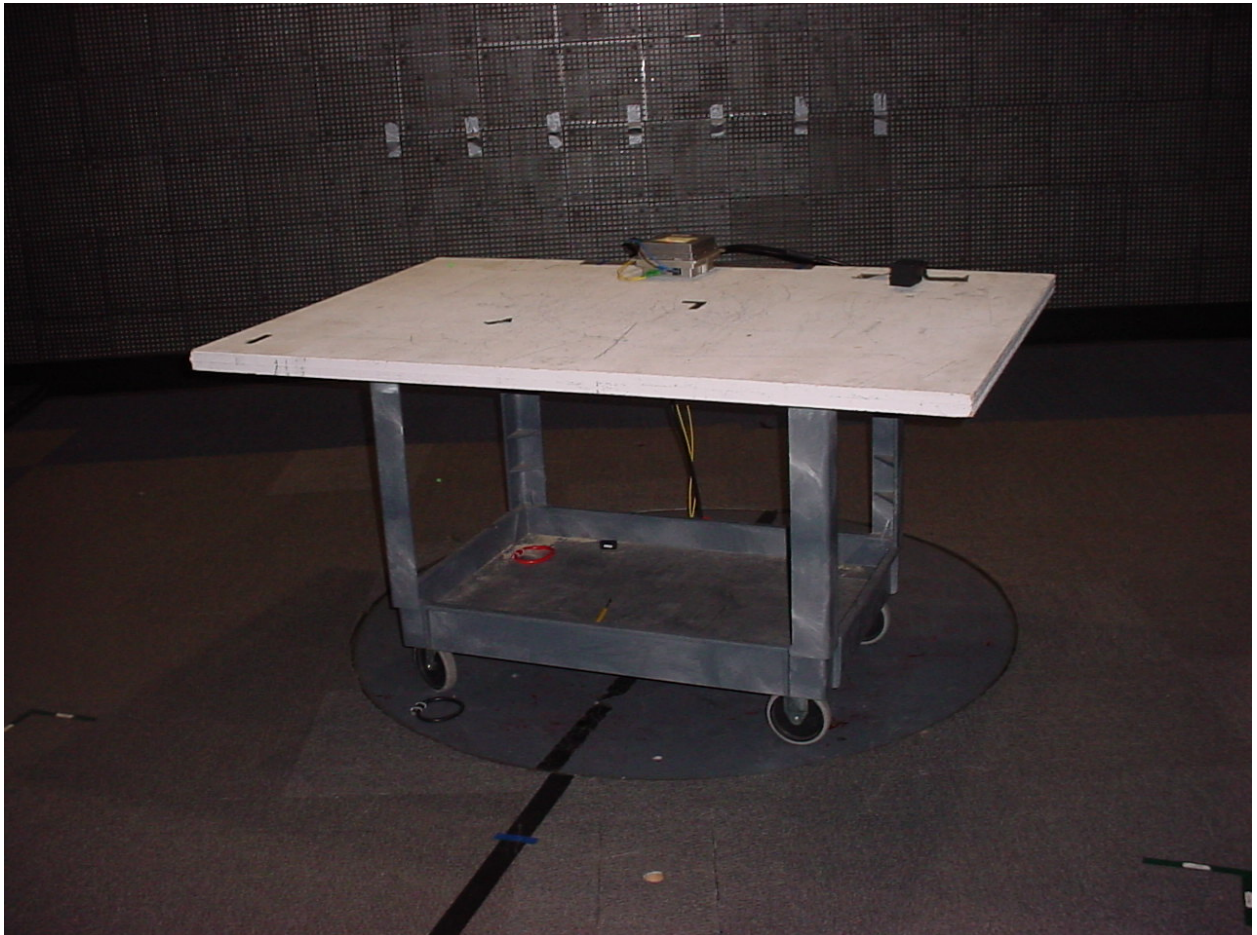
Figure 4: Test Setup – Radiated Emissions - Unintentional
