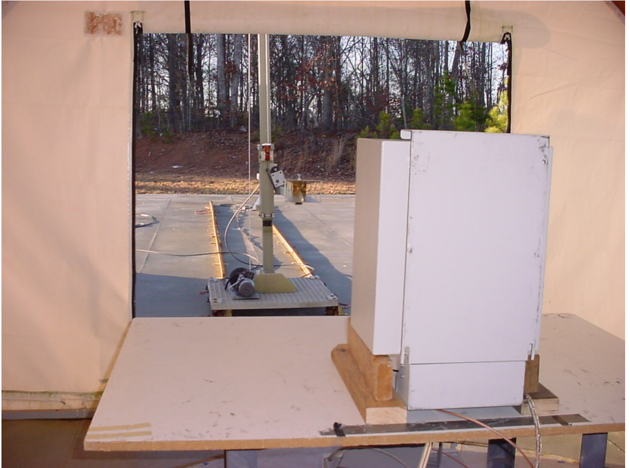
Figure 2: Test Setup - Radiated Emissions - Intentional
