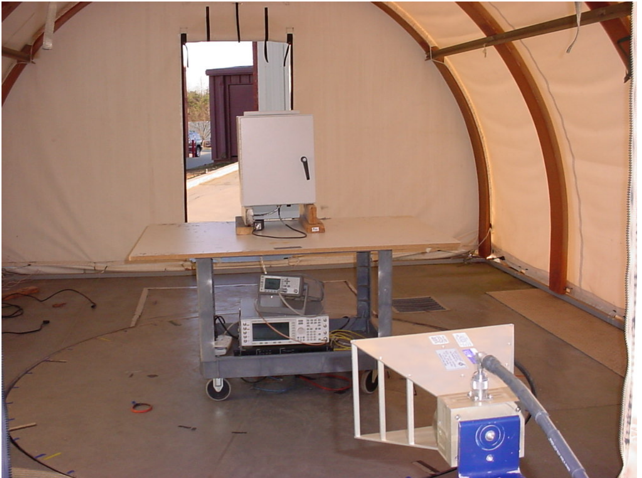
Figure 1: Test Setup - Radiated Emissions - Intentional
