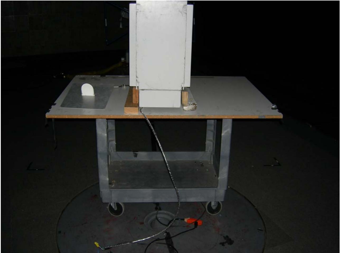
Figure 4: Test Setup - Radiated Emissions - Unintentional
