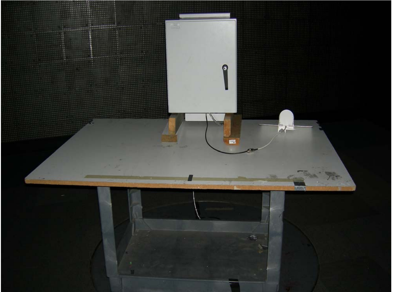
Figure 3: Test Setup – Radiated Emissions - Unintentional
