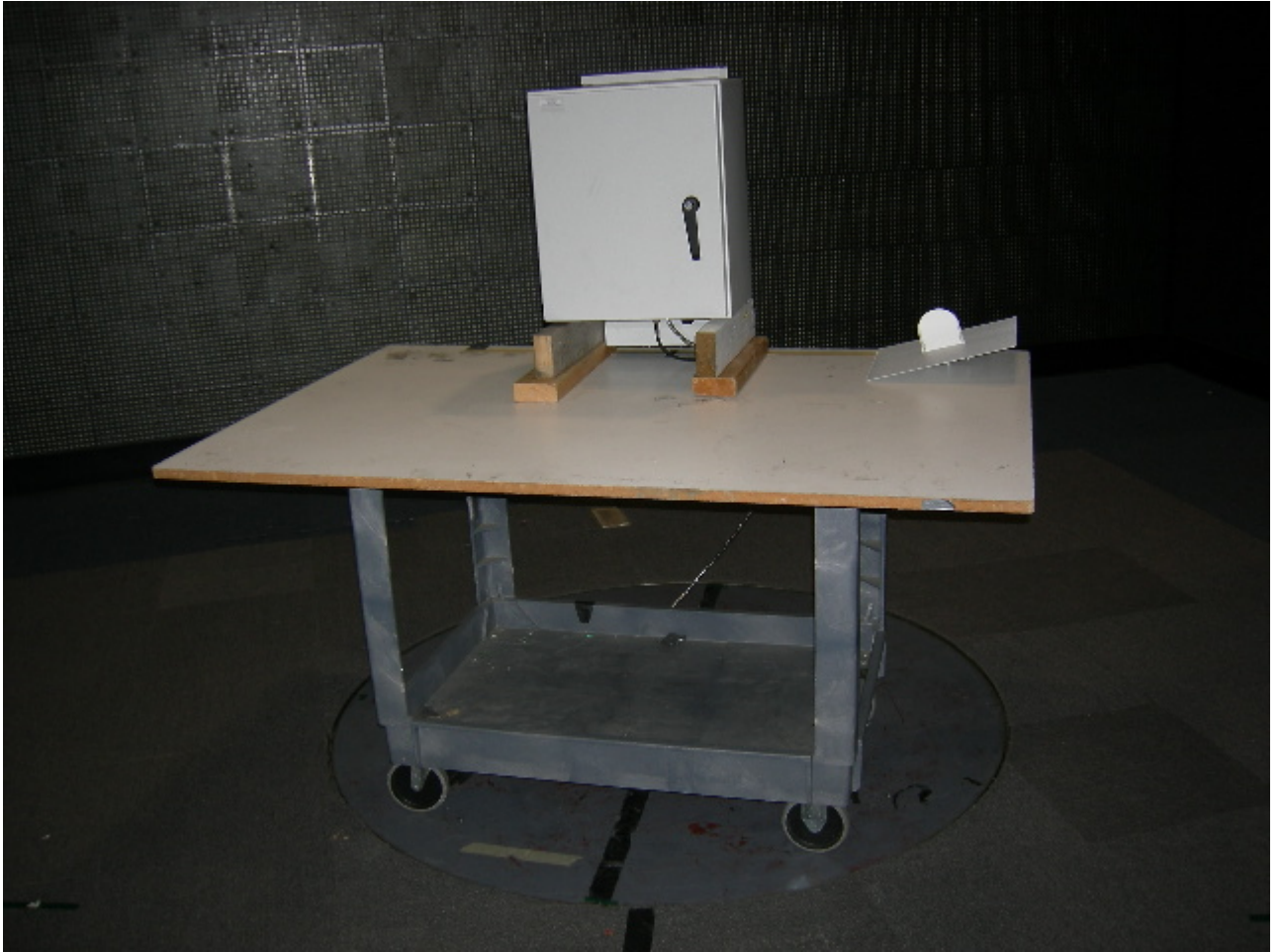
Figure 3: Test Setup – Radiated Emissions - Unintentional
