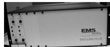
Typical EkoLink Plus Hub front panel shown with two RF/Optical Transceivers Installed
