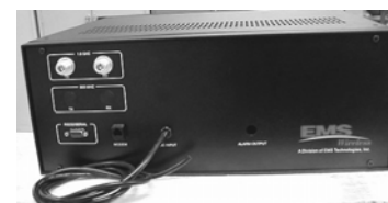
Typical EkoLink Plus Hub Rear Panel with 1900 MHz only
