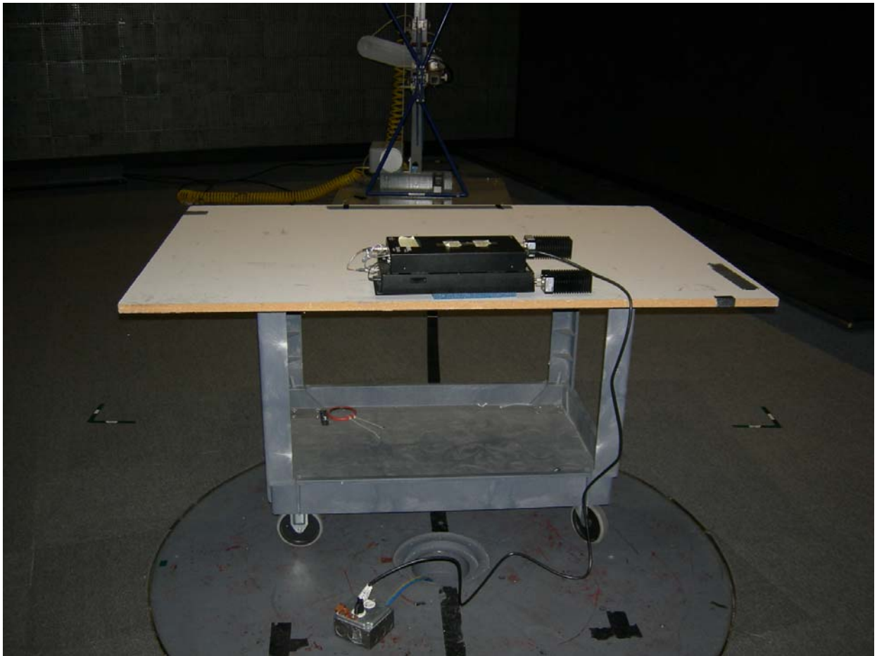
Figure 3: Test Setup – Radiated Emissions - Unintentional
