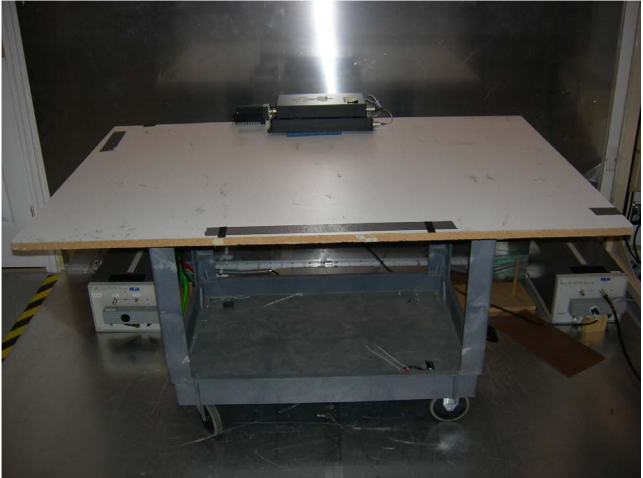
Figure 4: Test Setup – Power Line Conducted Emissions
