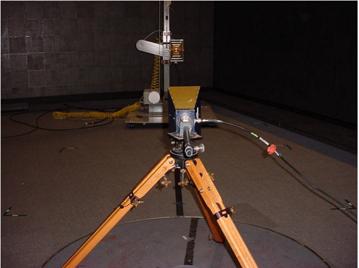
Figure 2: Test Setup – Radiated Spurious Emissions - Substitution
