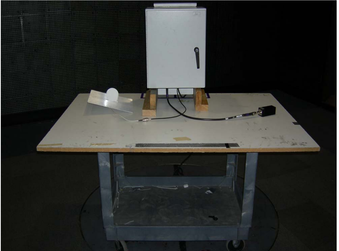
Figure 3: Test Setup – Radiated Emissions - Unintentional
