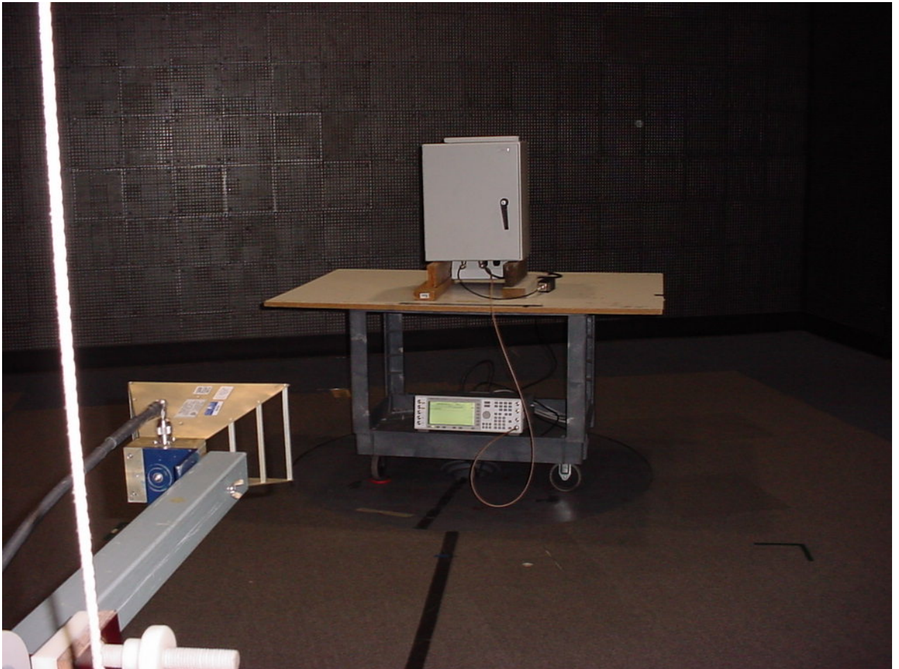
Figure 1: Test Setup - Radiated Emissions - Intentional
