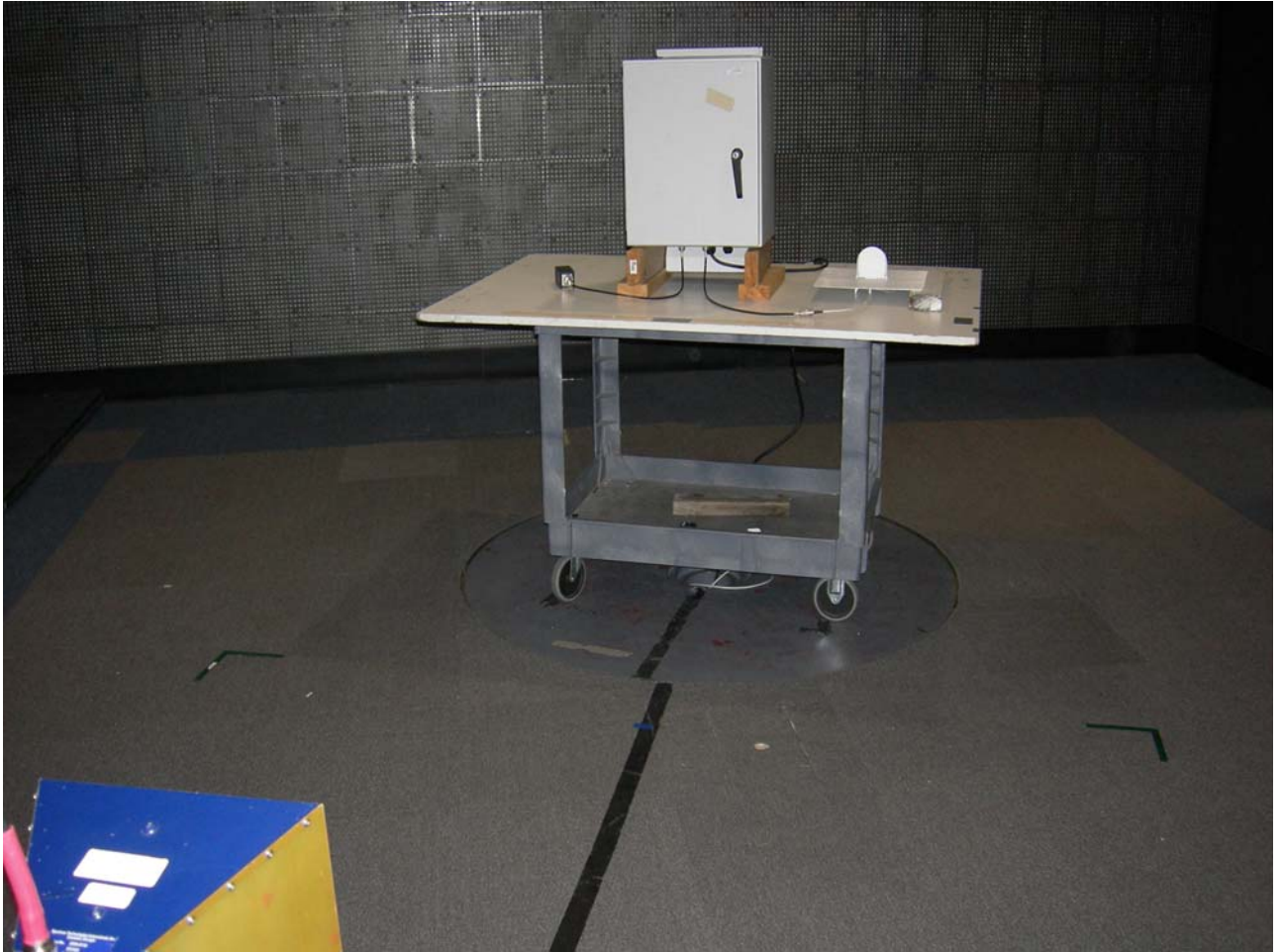
Figure 3: Test Setup – Radiated Emissions - Unintentional
