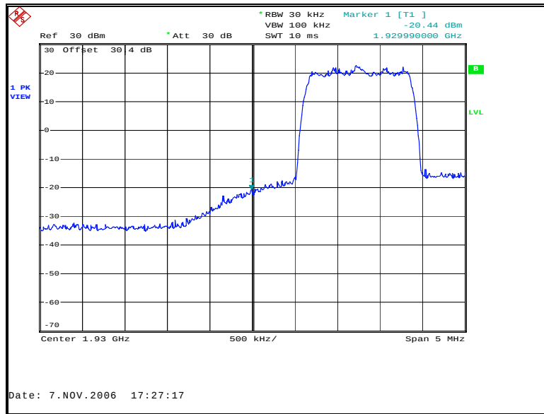
Figure 81: Band-Edge Downlink CDMA Low Channel
