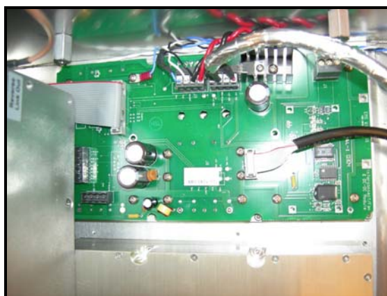
Figure 1.4-3 – Internal Photographs – Foil Wrapped Cable at DC Interconnect PCB
