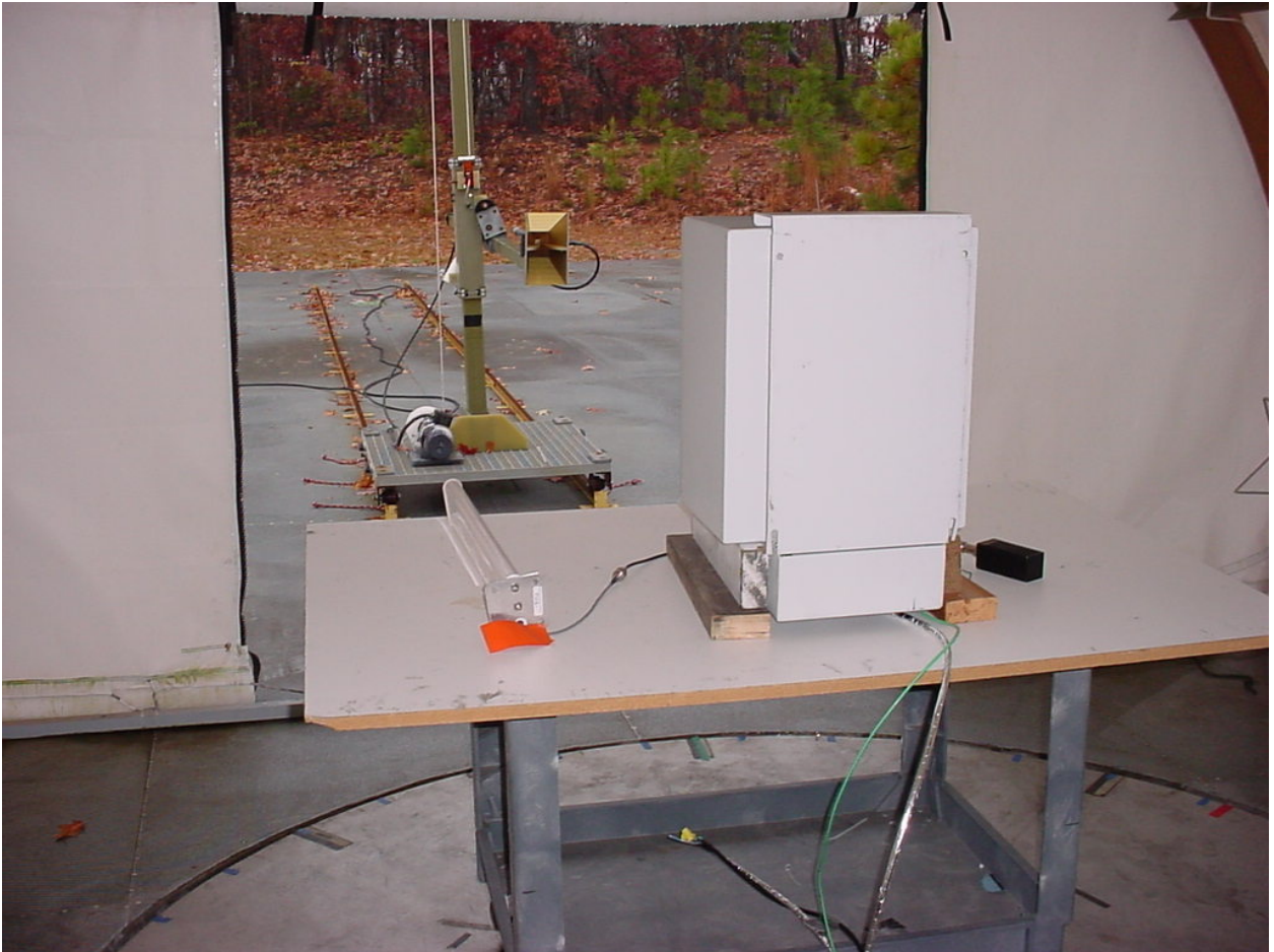
Figure 4: Test Setup - Radiated Emissions - Unintentional
