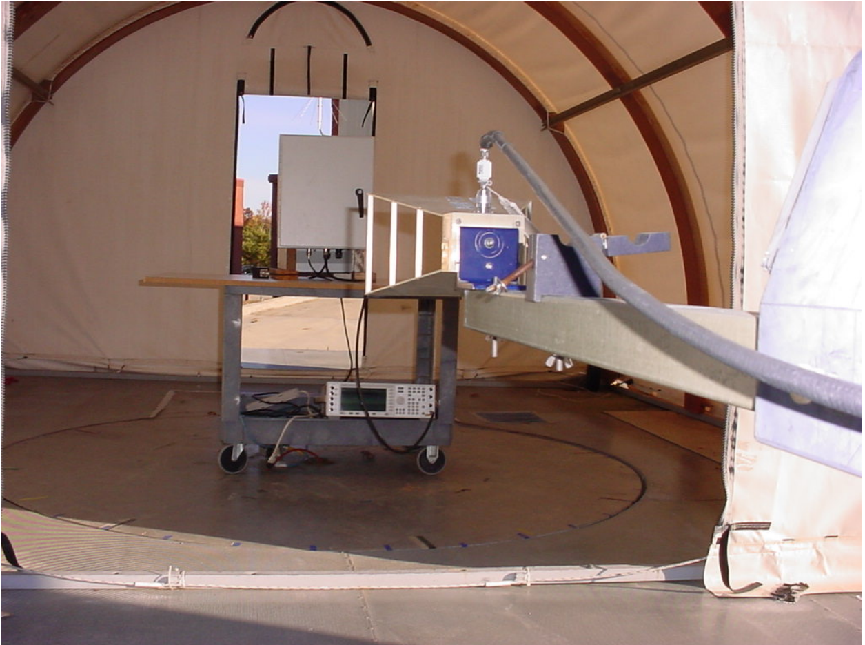
Figure 2: Test Setup - Radiated Emissions - Intentional
