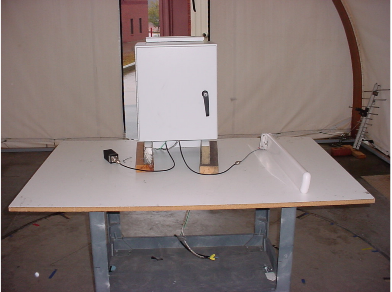
Figure 3: Test Setup – Radiated Emissions - Unintentional
