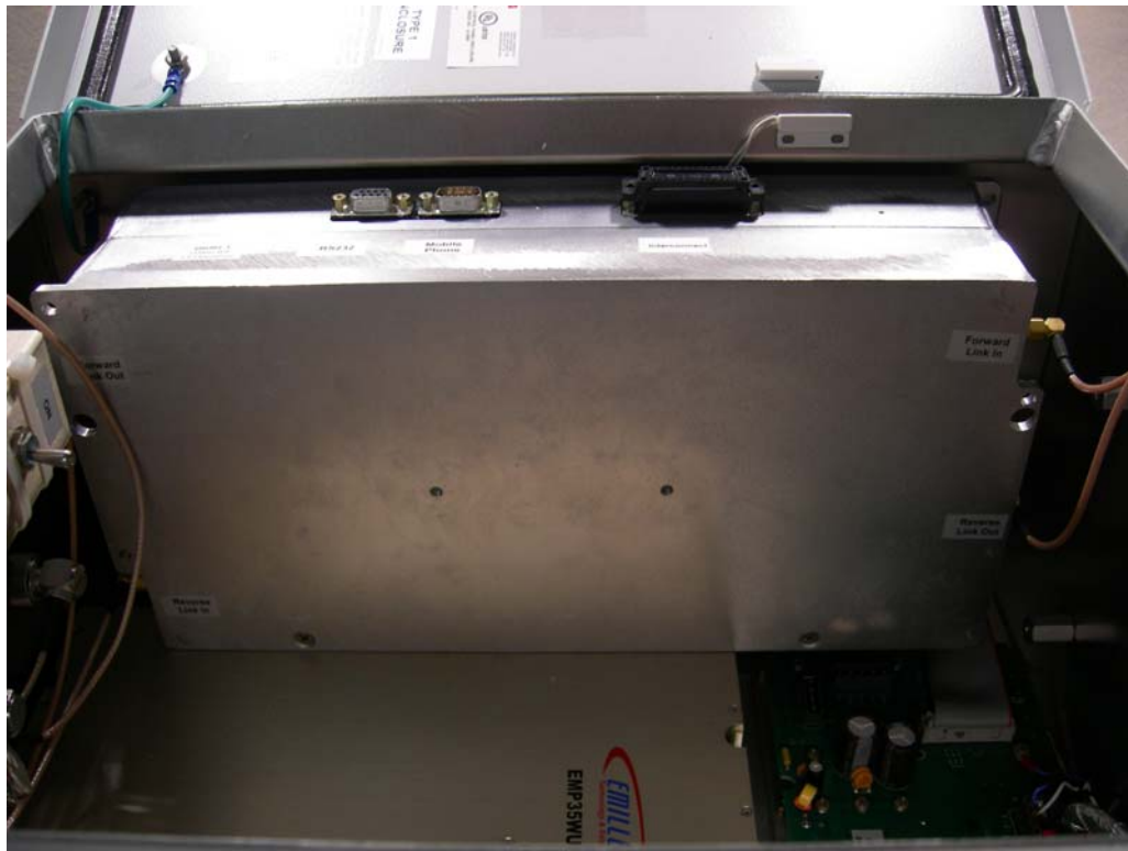
Figure 3: Internal – Assembled View - Channelizer
