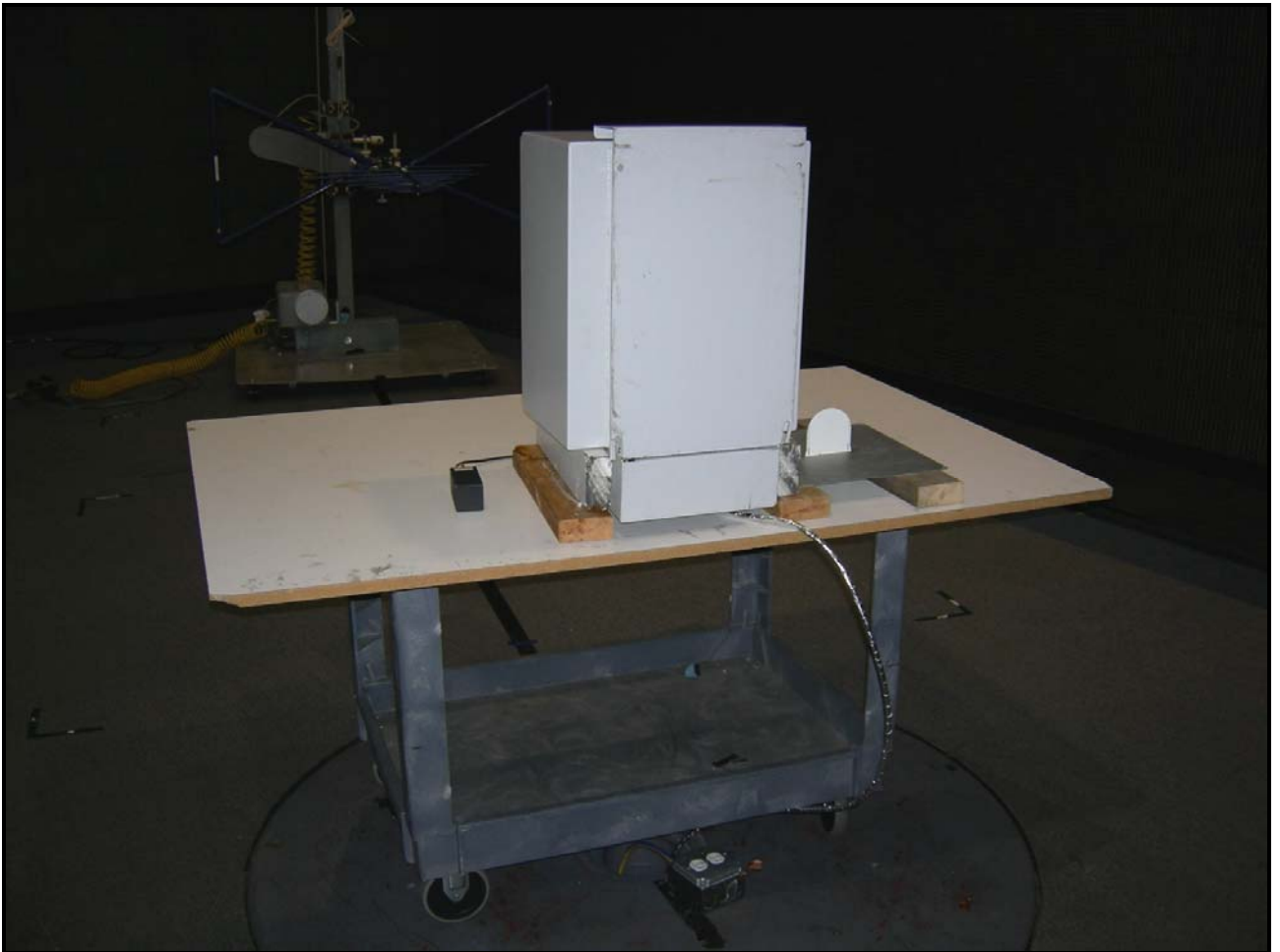
Figure 4: Test Setup - Radiated Emissions - Unintentional
