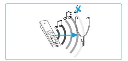
The range of the transmitter largely depends on environmental conditions such as wall thickness, wall composition etc. If the headphones leave the range of the transmitter, the audio first cuts out occasionally until it finally cuts out completely. You hear alerts in the stethoset receiver and the *Receiver status* LED flashes green (or red if the rechargeable battery is almost empty).
