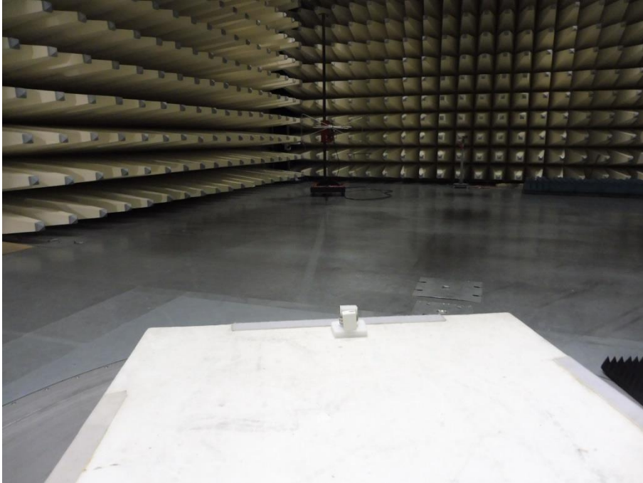
Photo 5: RSE set-up (30MHz to 1GHz)
