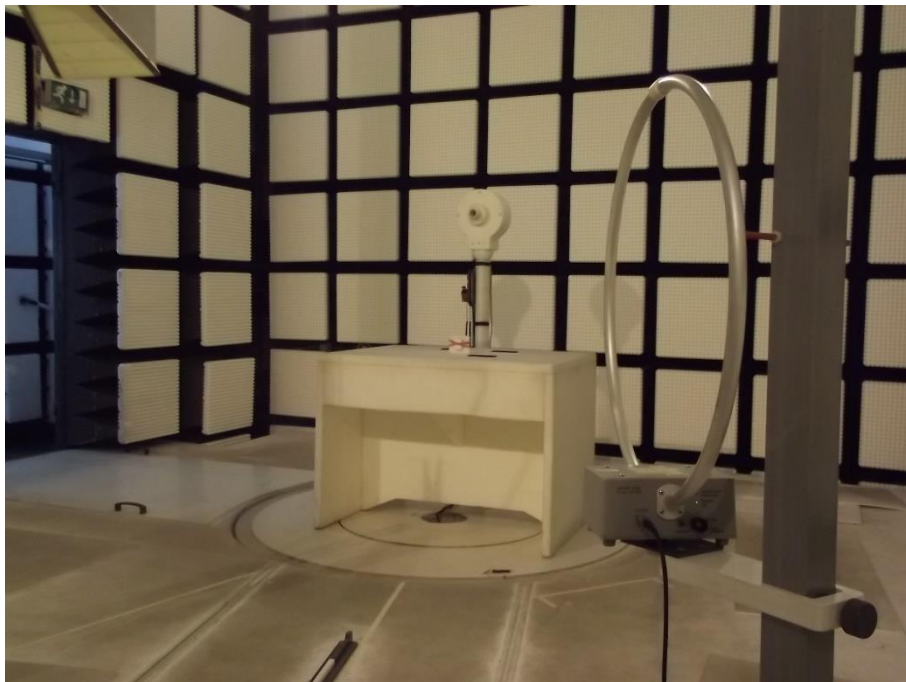
Photo 8: RSE set-up (<30MHz)
