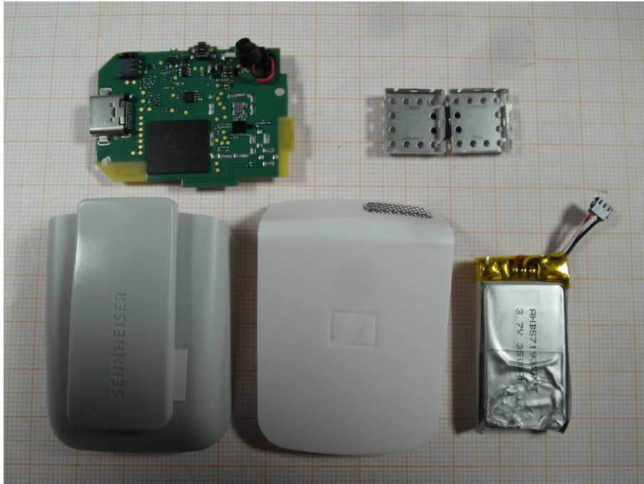
Photo 1: EUT disassembled with battery pack (front view)
