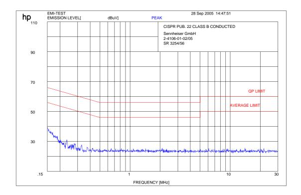
Upper Limit LINE CISPPR 22 QP Lower Limit LINE CISPPR 22 AV
